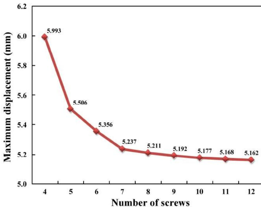
Fig. 6: The displacement versus number of screws in twelve-hole locked compression plate.
