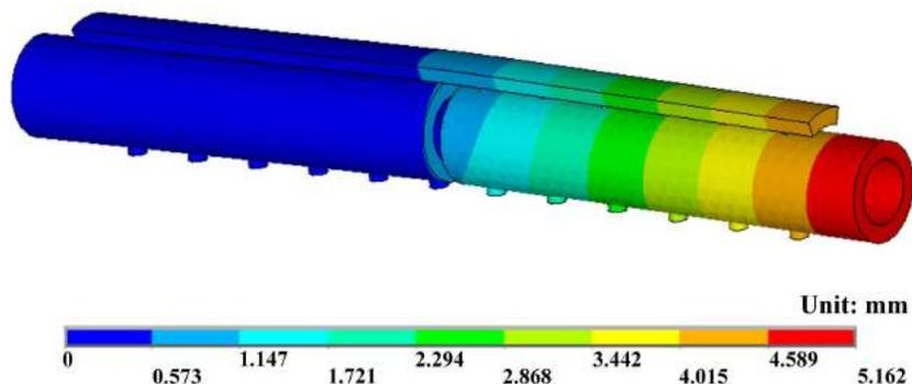
Fig. 3: Displacement distribution of the locked compression plate.
