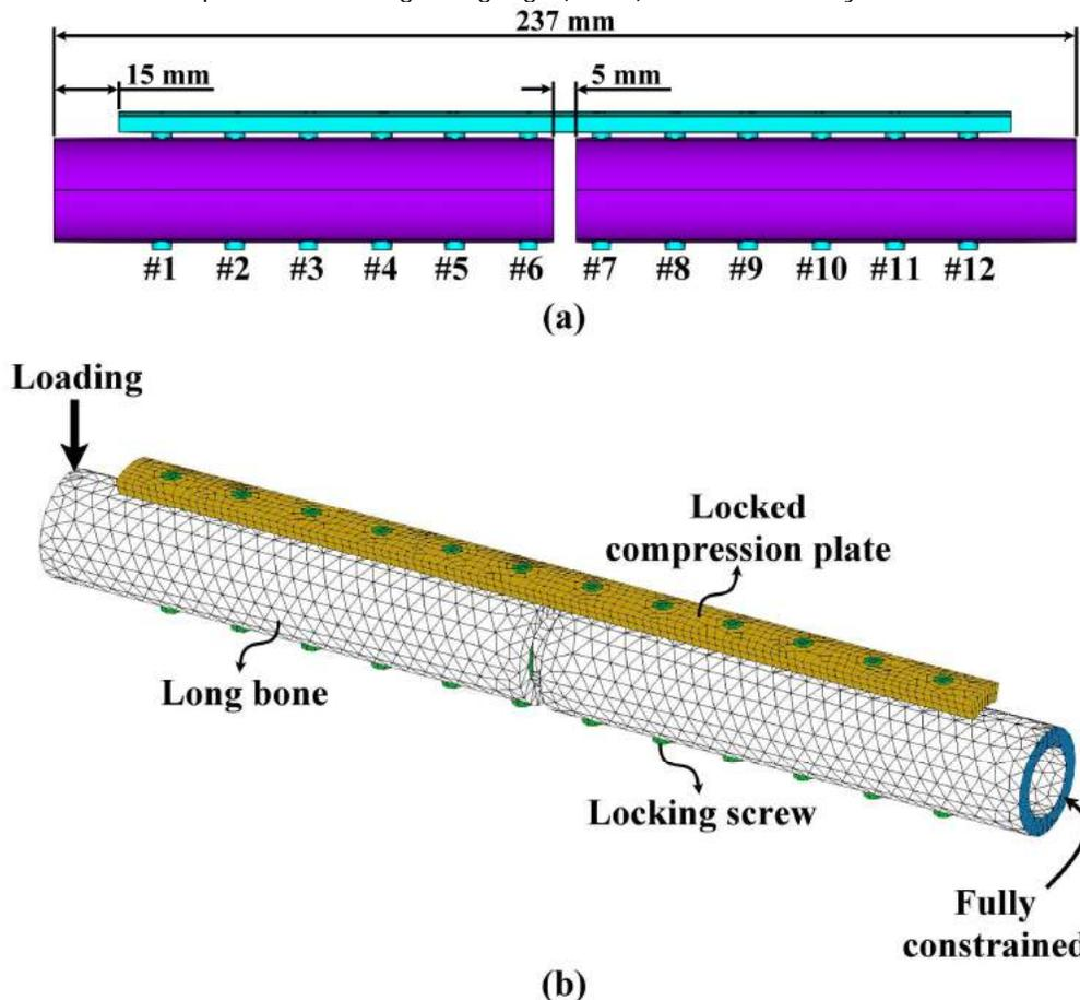
Fig. 1: The numerical models developed in this study: (a) Geometry and dimension, (b) Loading and boundary conditions.
