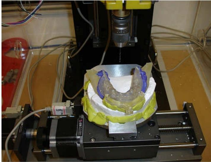
Fig. 9: Mandible model and surgical guide fixing on the drill press after indexing and origin locating.
