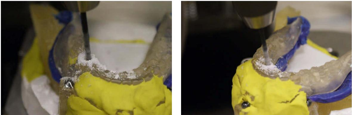
Fig. 10: Drill #45 (left) and #41 (right) holes on the 5-axis CNC drill press.
