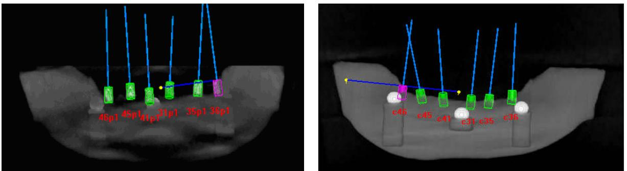
Fig. 13: CT-scanned images: (a) 5-axia CNC drilled model (left) and (b) Implantmed drilled model (right).
