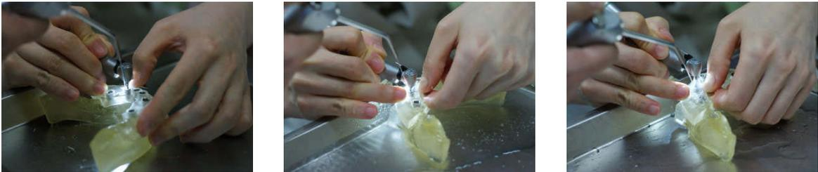
Fig. 12: Sequences of surgery simulation to drill #35 hole: (a) Drilling by 2.1mm drill (left), (b) Drilling by 2.5mm drill (middle), and (c) Drilling by 3mm drill (right).
