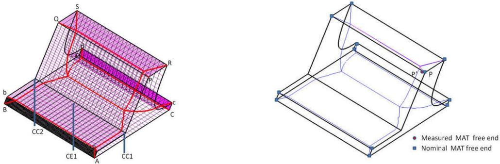
Fig. 5: (a) Nominal 'T' shape model with MAT (b) Measured perturbed 'T' shape model with nominal and measured MAT.
