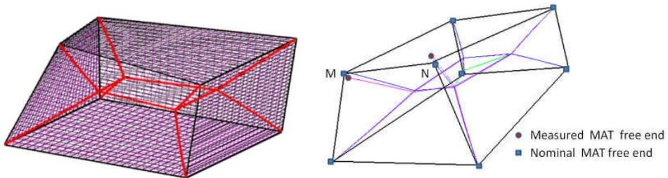
Fig. 4: (a) Nominal trapezium model with MAT (b) Measured Trapezium model with nominal and measured MAT.
