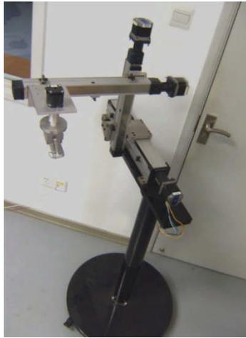
Fig. 3: The photo of the robot.
