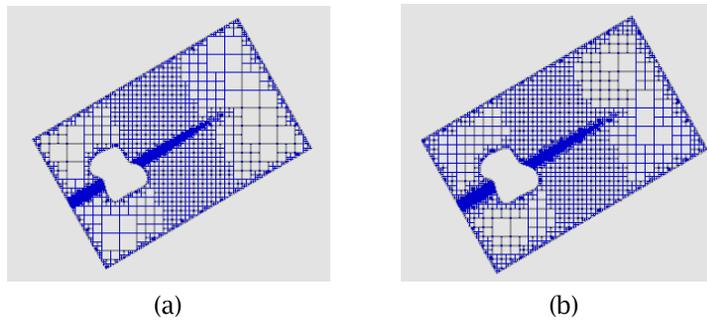
Fig. 11: (a) Material quadtree of  $H_2$ . (b) The balanced counterpart.
