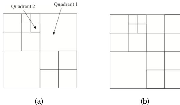
Fig. 8: An unbalanced quadtree and its balanced counterpart. (a) Quadrant 1 is greater than its neighbor quadrant 2 by four times and this quadtree is an unbalanced one. (b) The quadtree is balanced by subdivided quadrant 1.
