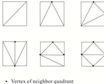
Fig. 9: Six plausible patterns to triangulate a Homo quadrant (the other patterns can be retrieved using the rotational symmetry properties) [6].
