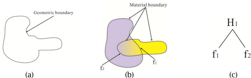
Fig. 2: (a) A 2D geometric model. (b) A heterogeneous model  $H_1$ . The boundaries of the object are called material boundaries. (c) The HFT of  $H_1$ .
