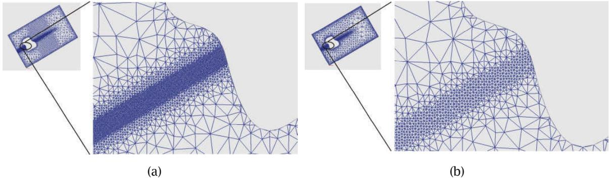
Fig. 14: (a) Comparison of meshes with different thresholds. (a) Quadtree resolution = 7, material composition variation threshold = 0.1 (b) Quadtree resolution = 7, material composition variation threshold = 0.2
