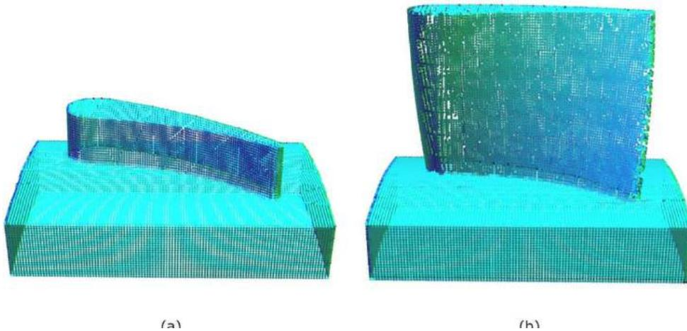
Fig. 9: Shape editing for a point cloud corresponding to a turbine blade that is extended and twisted such that the center of gravity of each horizontal cross section remains along a vertical line.
