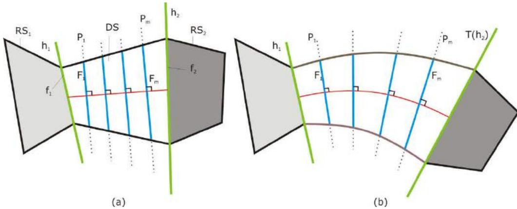
Fig. 3: Splitting a solid with two planar separating surfaces  $h_1 \neq h_2$ , which results into a deformable subset  $DS \neq \emptyset$  and in two generally non-congruent faces  $f_1$  and  $f_2$ ; the computed cross-sections shown in (a) are repositioned in (b) according to the prescribed deformation.
