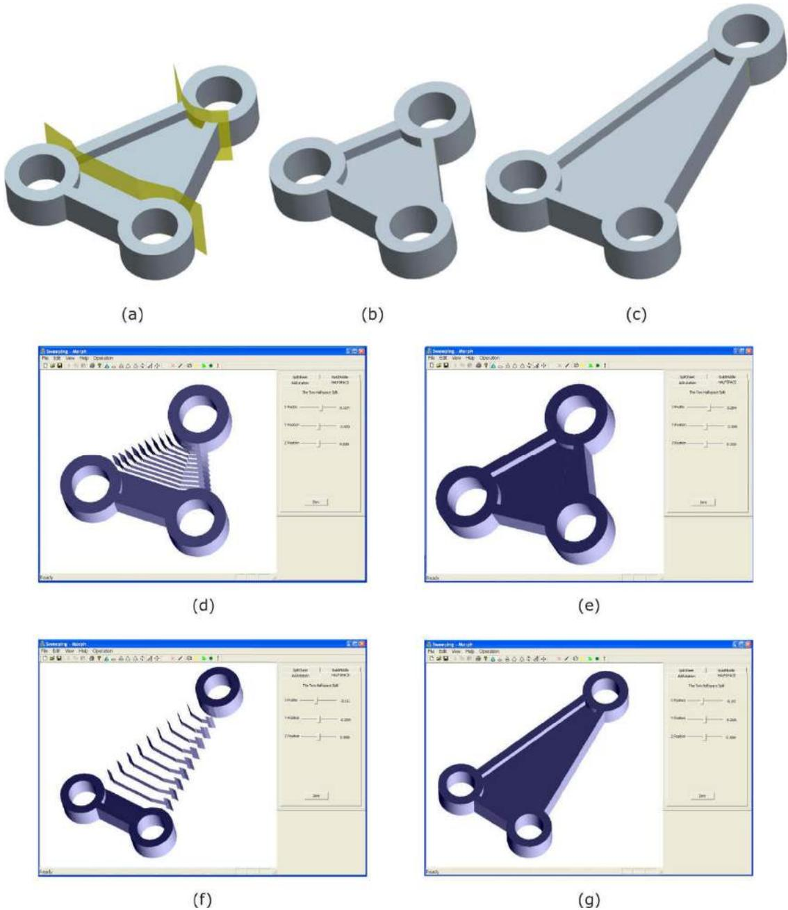
Fig. 13: The shape of Figure 11, illustrated in (a), is shrunken in (d) and (e), and extended in (f) and (g) with continuity by using piecewise linear separating surfaces (a). The resulting shapes are also shown in (b) and (c).
