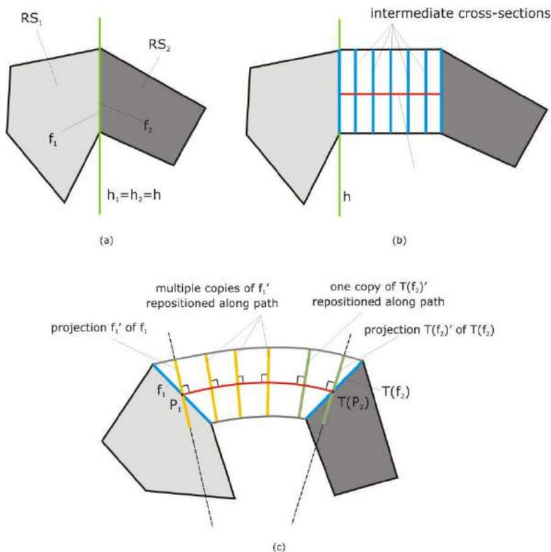
Fig. 2: (a) Splitting a solid with one planar separating surface (i.e.,  $h_1 = h_2$ ), which results in an empty deformable subset  $DS = \emptyset$ , and two new identical faces  $f_1$  and  $f_2$ ; (b) illustrates the stretching of the original part; (c) shows a more general deformation for Case 1.
