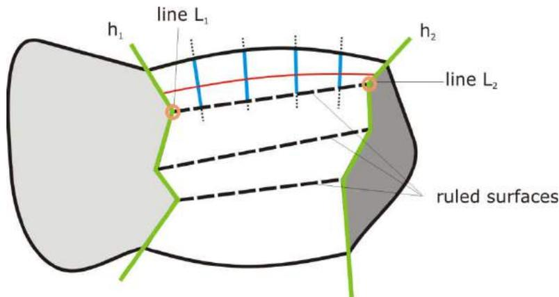
Fig. 4: If the two separating surfaces are piecewise linear having the same number of planar segments, the problem reduces to either the one shown in Figure 2 or Figure 3 for each pair of planar segments depending on whether the two separating surfaces are identical or not.
