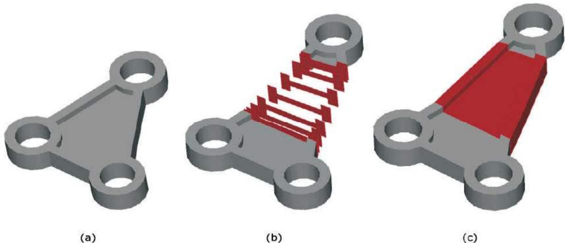
Fig. 11: A local scaling deformation with varying cross-section which points out one problem that can arise from an improper choice of the separating surfaces. Note the loss of smoothness between some of the newly created faces and the old faces of the part.
