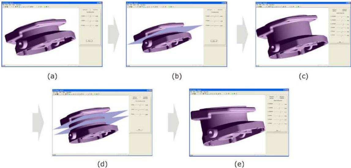
Fig. 7: Two successive deformations applied on a molded part: the stretching illustrated in Figures (b) and (c) is followed by the bending deformation shown in (d) and (e).
