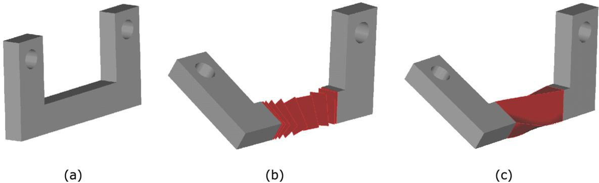
Fig. 6: A twisting shape deformation with constant cross-section and constrained total length is obtained by splitting the original geometry with two planar separating surfaces and generating the corresponding deformed geometry as proposed in section 2.
