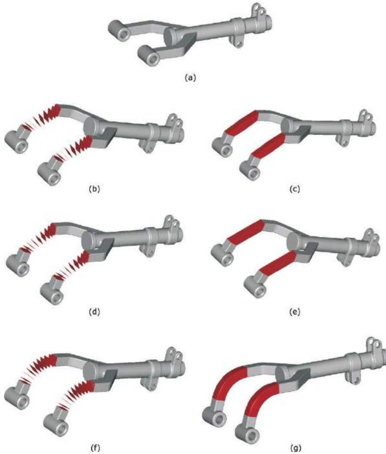
Fig. 5: A bending shape deformation with or without constant cross-section using one planar separating surface. The original geometry is shown in (a), while the pairs of figures (b) & (c), (d) & (e), and (f) & (g) show different resulting shapes depending on the key configurations prescribed. In figures, (e) and (g) the constant cross-section of the generated geometry is preserved.
