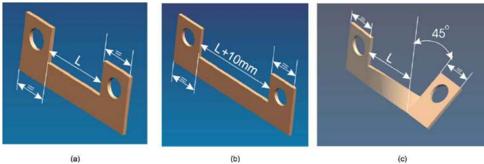
Fig. 1: Three simple brackets those are geometrically similar. Current CAD systems support parametric models that can change bracket (a) to (b), but not bracket (a) to (c) because bracket (c) is not in the same “parametric family” [33] with brackets (a) and (b).
