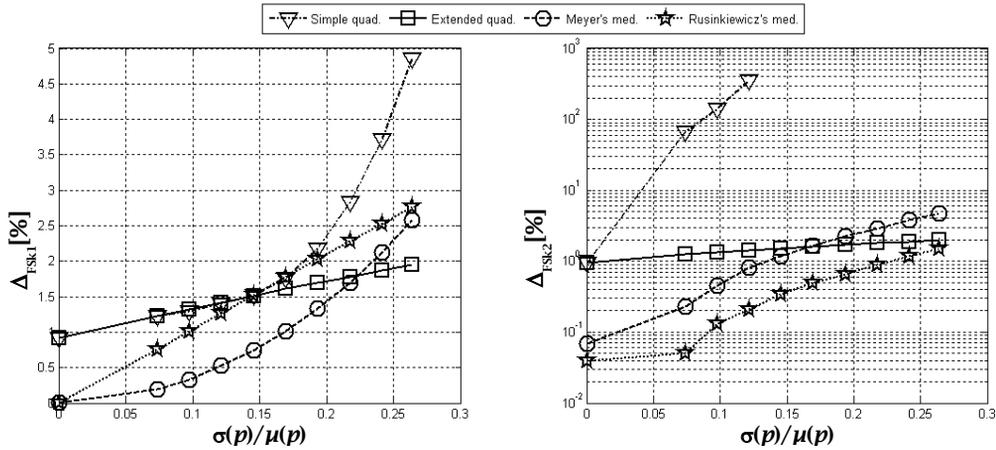
Fig. 10. Impact of  $\sigma(p)/\mu(p)$  on the error in the estimated focal points' location (tessellated torus:  $\mu(p)H = 0.06, n_v(p)=6$ ).
