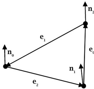
Fig. 4. Edges and normal directions used in the Rusinkiewicz's method [27] to build the *curvature tensor* of a triangle.
