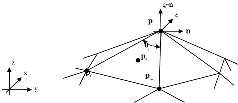
Fig. 3: Piecewise-linear surface and the local coordinate system  $(\xi, \psi, \zeta)$ .
