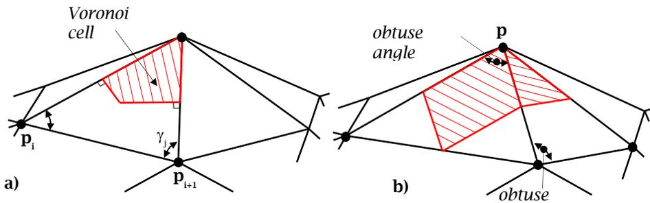
Fig. 1: The *Voronoi cell* (a) and the integration cells (b) associated, respectively, to a non-obtuse triangle and to the two different typologies of obtuse triangles of the  $1$ -ring neighborhood of  $\mathbf{p}$ .
