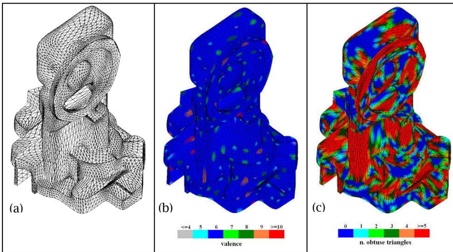
Fig. 13. Quality of the mesh (valence (b) and obtuse triangles (c)) of a typical mesh of a scanned object (a).
