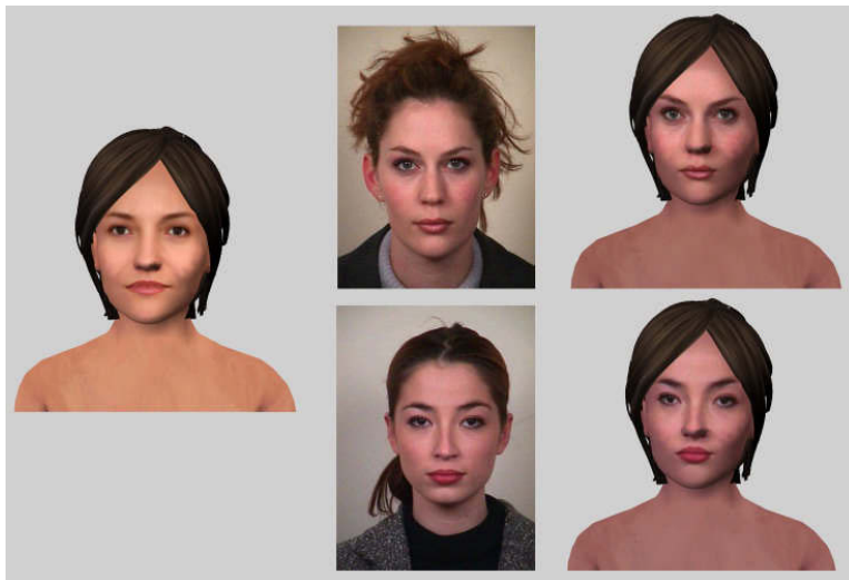
Fig. 5: Starting from a template avatar and based on a user's photo, avatars are personalized through a face detection based retexturing of the body.
