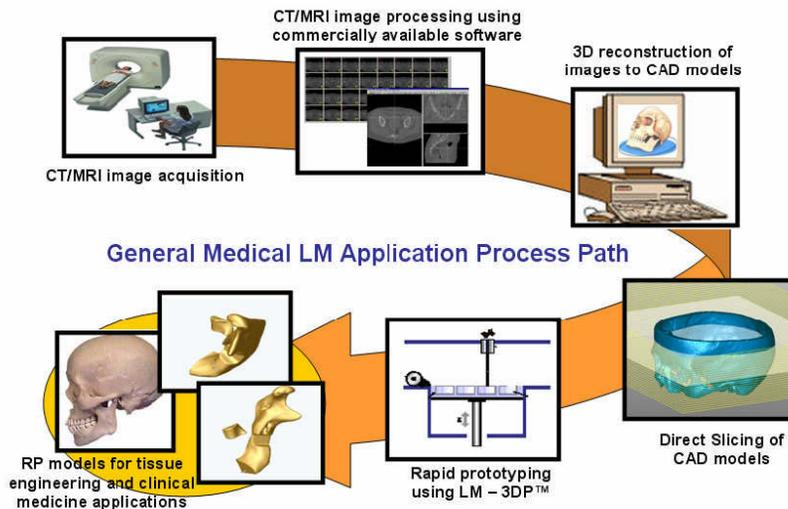
Fig. 1: General biomodeling and medical rapid prototyping process path.
