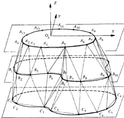
Fig. 3: Method of planar contours.
