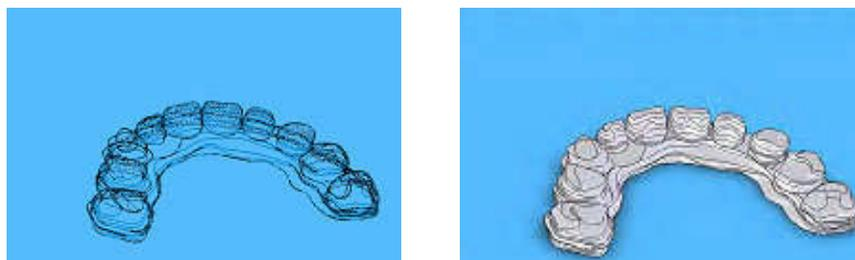
Fig. 6: (a) Layers closed curves selected for a loft feature, (b) Solid model by planar contours method.
