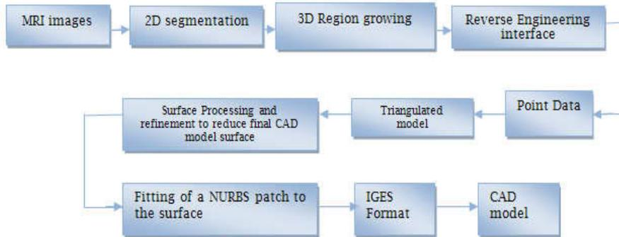
Fig. 2: Process definition to arrive at a CAD model from CT and MRI data.
