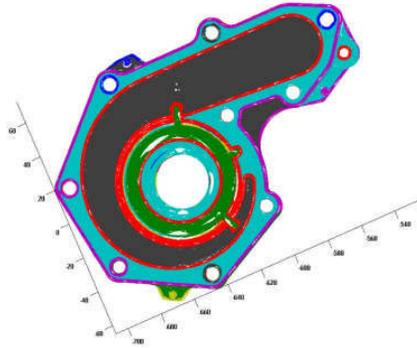
Fig.10: Geometrical feature segmentation of the pump carter.
