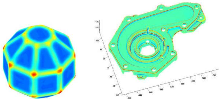
Fig. 4: (a) Curvatures of a 26-face polyhedron-measuring artefact, (b) curvature of a pump carter.
