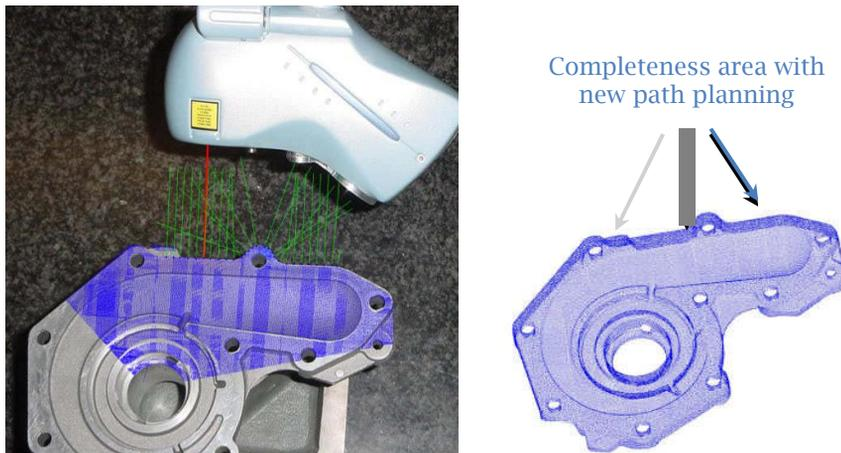
Fig.7: (a) new path planning simulation, (b) the actual final points cloud generated by the application of the 3D intelligent path planning.
