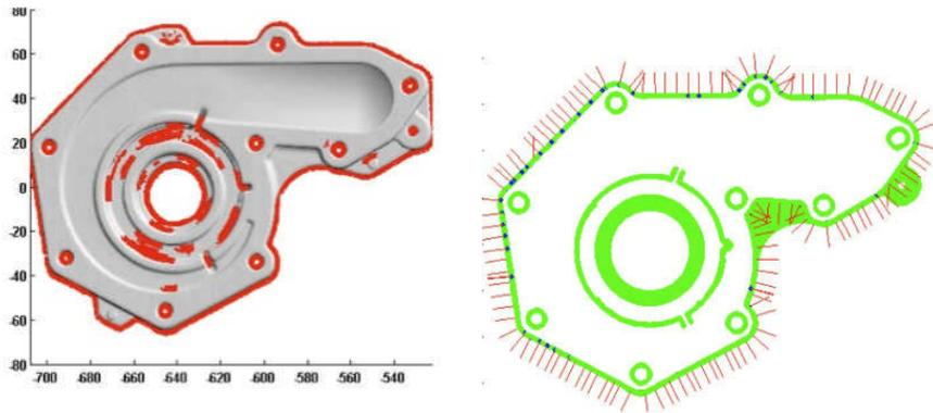
Fig. 6: Results of the Scale Space Algorithm: (a) Characteristic line extraction, (b) Normal evaluation for the outside borderline.
