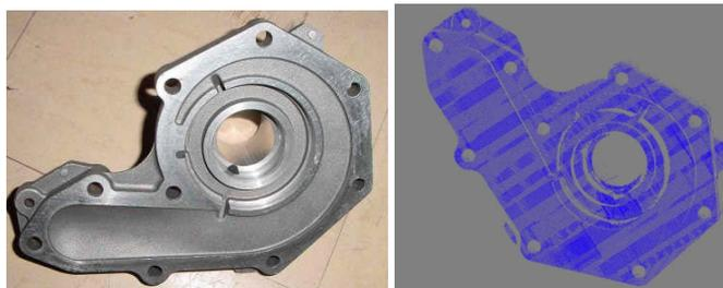
Fig. 5: Illustrated case: (a) pump carter, (b) first digitizing cloud of points.
