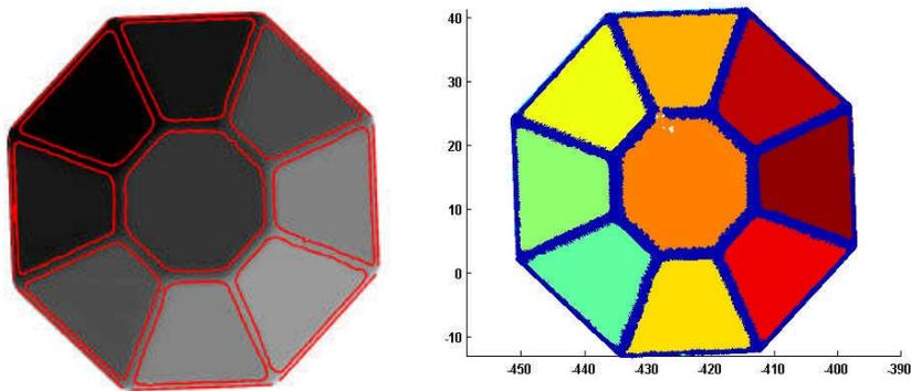
Fig. 9: (a) extraction of level line 0.12 of a spherical faced measurement artefact, (b) segmentation in flat and non-flat zones.
