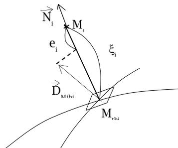
Fig. 11: Distances between the scanned point and the theoretical point.
