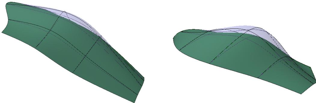
Fig. 8: (a) 5% increase in area freely moving 6CPs; (b) modified surface (blue) and original (green).
