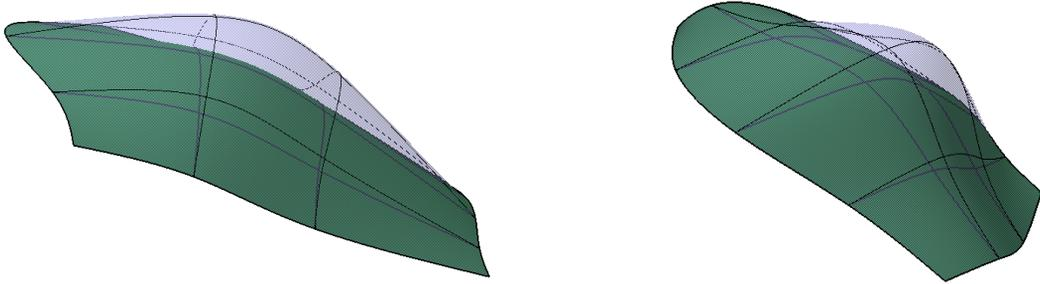
Fig. 7: (a) 10% increase in area moving Z-coords of 6CPs; (b) modified surface (blue) and original (green).
