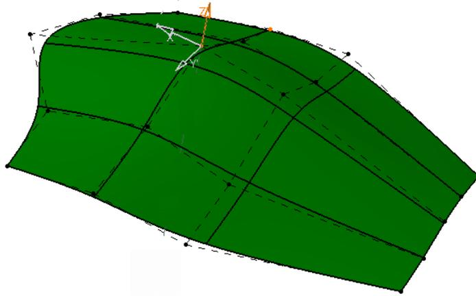
Fig. 4: Canopy surface; original area:  $5014.36\text{m}^2$ ; dashed lines show control mesh.
