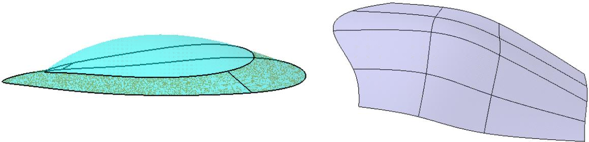
Fig. 2: CAD surface models of (a) a domed skylight for a mall (b) a portion of the canopy of a hotel building.
