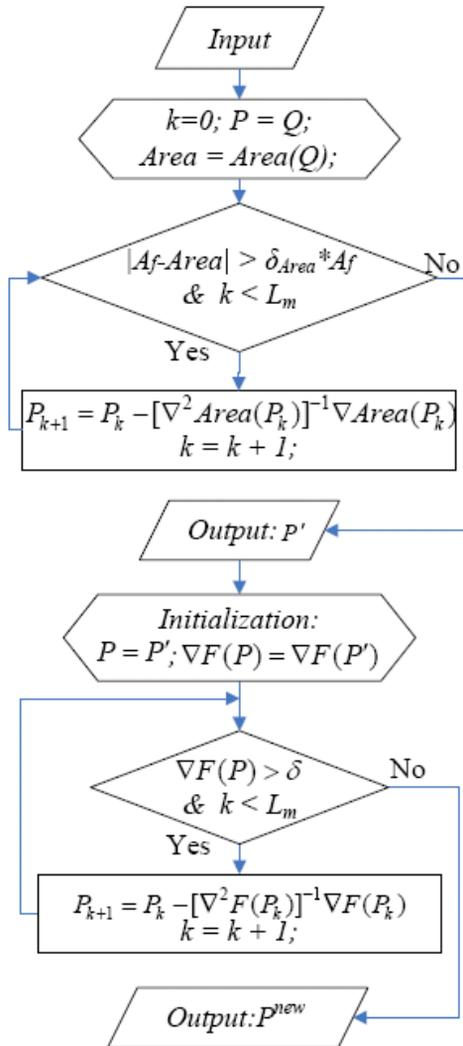
Fig. 3: The modified Newton’s approach for the constrained surface modification problem.
