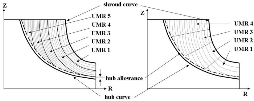
Fig. 2: Conventional rough cut plan (left) vs. proposed partitioning of a machining area (right).
