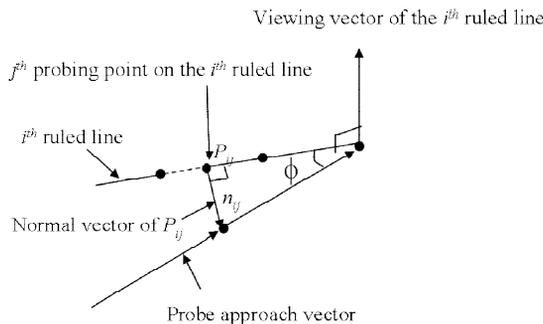
Fig. 8: Measuring point Pij and probe approach vector.
