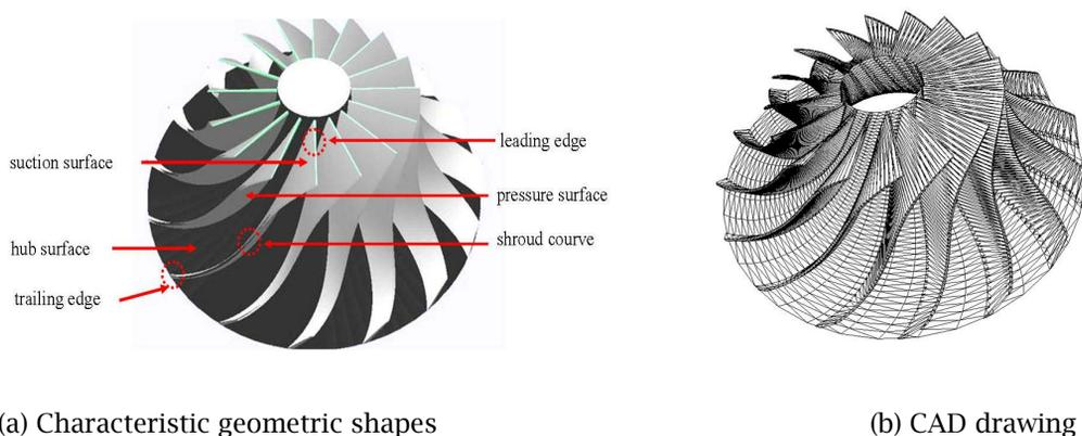
Fig. 1: Typical impeller configurations.
