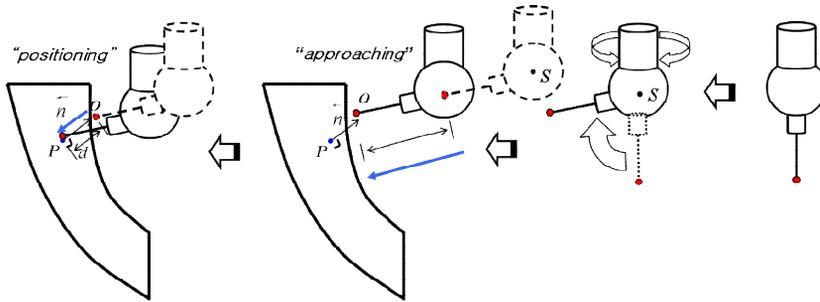
Fig. 7: A probe approach motion to a point of a blade surface.
