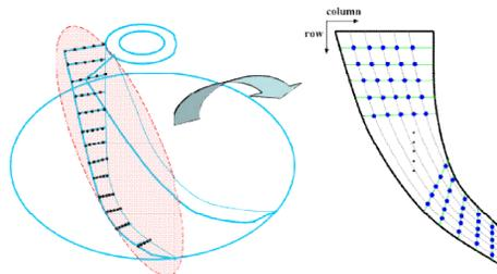
Fig. 6: Sampled measurement points on a blade surface of an impeller.
