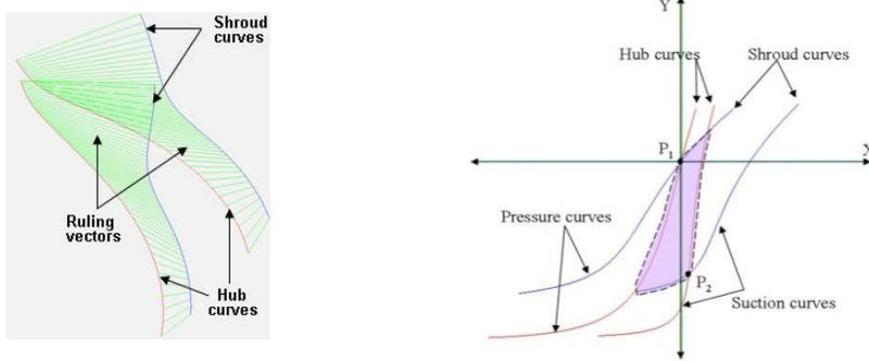
(a) ruling vectors of blade surfaces      (b) projected blade curves
