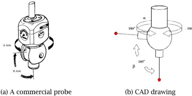
Fig. 5: A rotating and tilting probe.
