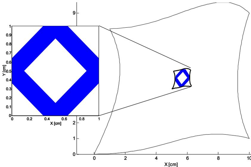
Fig. 4: Mapping a unit geometric primitive into subdivided region.
