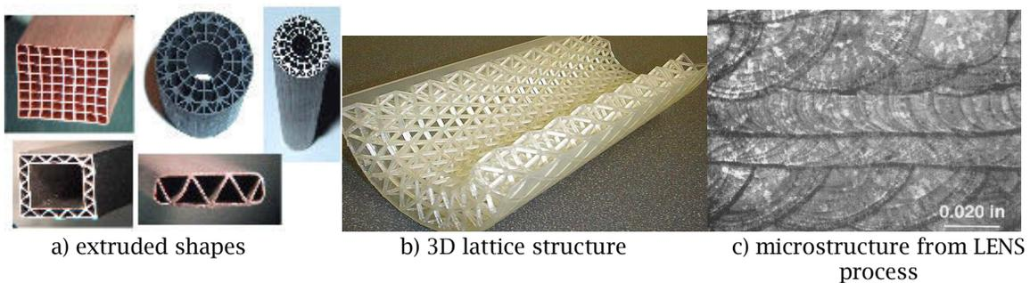
Fig. 1: Example cellular structures and additive manufacturing microstructure.
