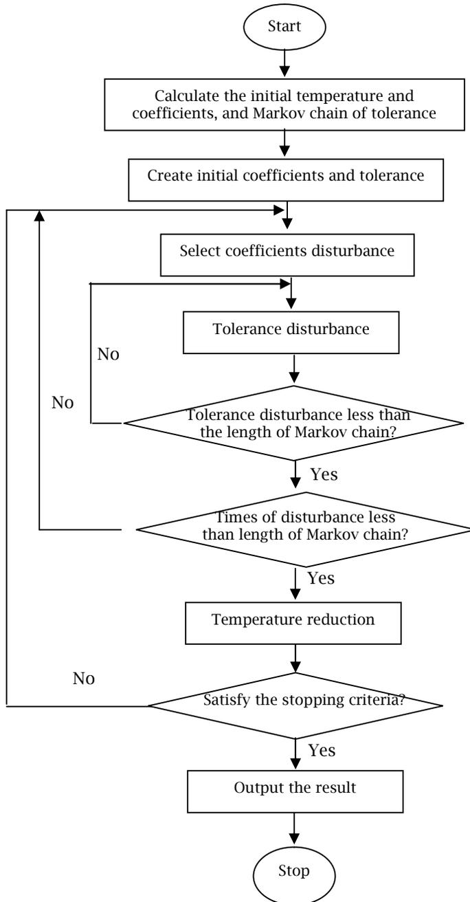
Fig. 2: Flow chart of tolerance design based on SA algorithm.
