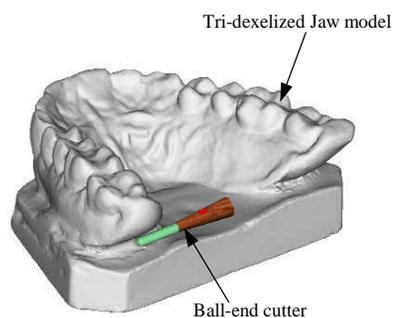
Fig. 11: Haptic virtual sculpting of a tri-dexel model.
