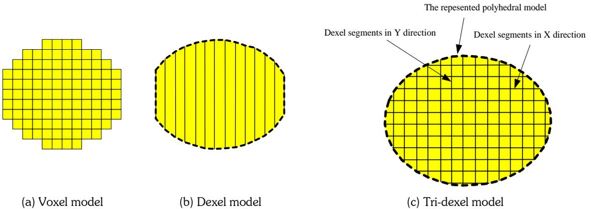
Fig. 1: Comparison of different volumetric modeling methods.
