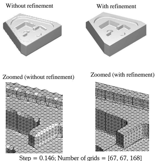
Fig. 9: Tri-dexel representation of a joystick base model.
