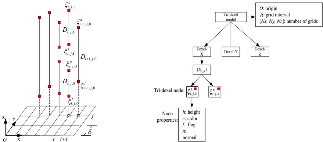
(a) Data structure of a dexel model (b) Hierarchical data structure
