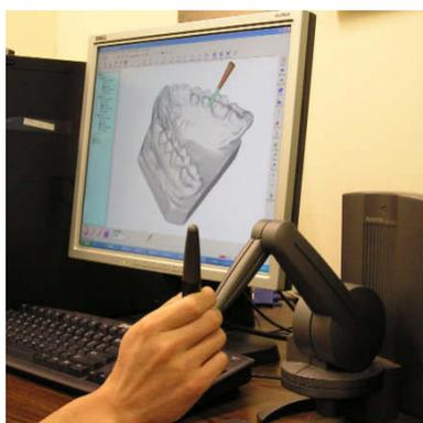
Fig. 10: A tri-dexel-based haptic virtual design system.
