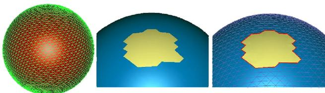
Fig. 3: Hole on a mesh model and the detected hole boundary.
