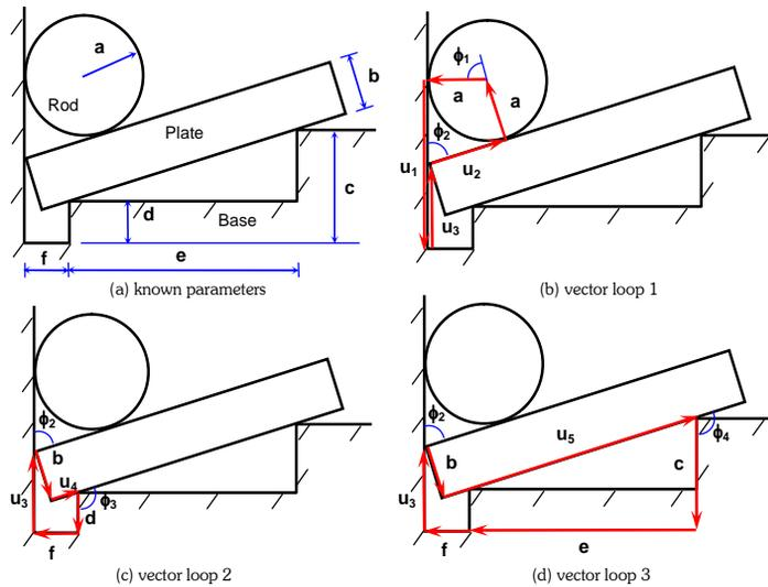
Fig. 6: A stacked block assembly with closed loops of variations.
