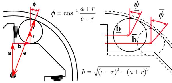
Fig. 1: An example of one-way clutch variation estimation.
