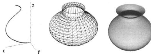
Fig. 2: Rotational Sweep: A profile curve, the surface of revolution, the shaded image [13].
