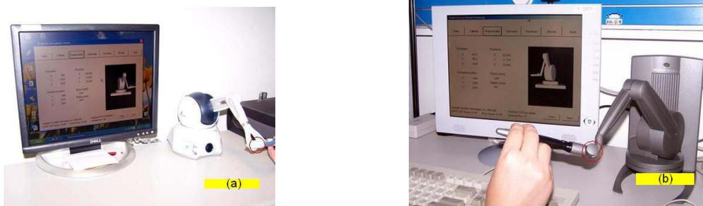
Fig. 1. SensAble PHANTOM® OMNI™ (a) haptic device and SensAble PHANTOM® DESKTOP™ (b) haptic device.
