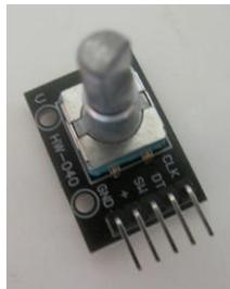
**Figure 6:** Rotary encoder KY-040.
