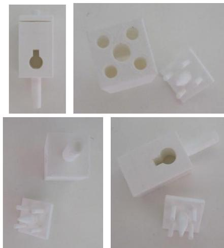
**Figure 11:** 3D printed button.
