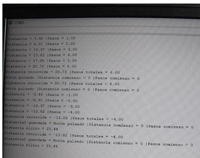
**Figure 7.** The first test of the rotary encoders with code programming on the Arduino UNO platform.
