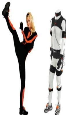
**Figure 1:** Xsens MVN motion capture system.
