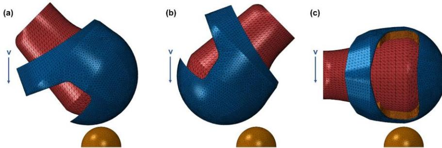
**Figure 3:** (a) Front, (b) back, and (c) right impact simulation configuration on spherical anvil.
