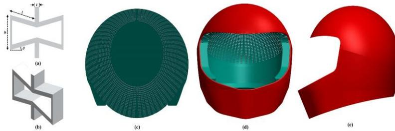
**Figure 2:** (a) Representation of an auxetic honeycomb unit cell, (b) Isometric view of the unit cell, (c) Top view of the helmet liner containing auxetic honeycomb pores, (d) Front view of the aux-pore liner helmet, (e) Side view of the helmet.
