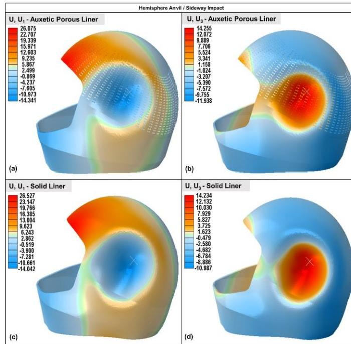
**Figure 7:** Comparison of  $u_1$  and  $u_3$  deformation between Aux-pore and solid liner when subjected to sideways impact configuration under hemispherical anvil (a)  $u_1$  deformation contour of the Aux-pore liner, (b)  $u_3$  deformation contour of the Aux-pore liner, (c)  $u_1$  deformation contour of the solid liner, (d)  $u_3$  deformation contour of the solid liner.
