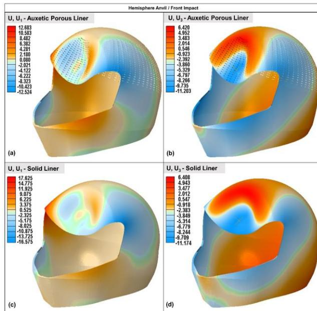
**Figure 5:** Comparison of  $u_1$  and  $u_3$  deformation between Aux-pore and solid liner when subjected to front impact configuration under hemispherical anvil (a)  $u_1$  deformation contour of the Aux-pore liner, (b)  $u_3$  deformation contour of the Aux-pore liner, (c)  $u_1$  deformation contour of the solid liner, (d)  $u_3$  deformation contour of the solid liner.
