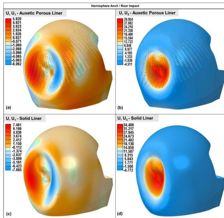
**Figure 6:** Comparison of  $u_1$  and  $u_3$  deformation between Aux-pore and solid liner when subjected to rear impact configuration under hemispherical anvil (a)  $u_1$  deformation contour of the Aux-pore liner, (b)  $u_3$  deformation contour of the Aux-pore liner, (c)  $u_1$  deformation contour of the solid liner, (d)  $u_3$  deformation contour of the solid liner.
