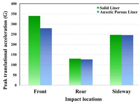
**Figure 8:** Comparison of the head form peak translational acceleration of the solid liner and the Aux-pore liner during three different impact configurations against the hemispherical anvil.
