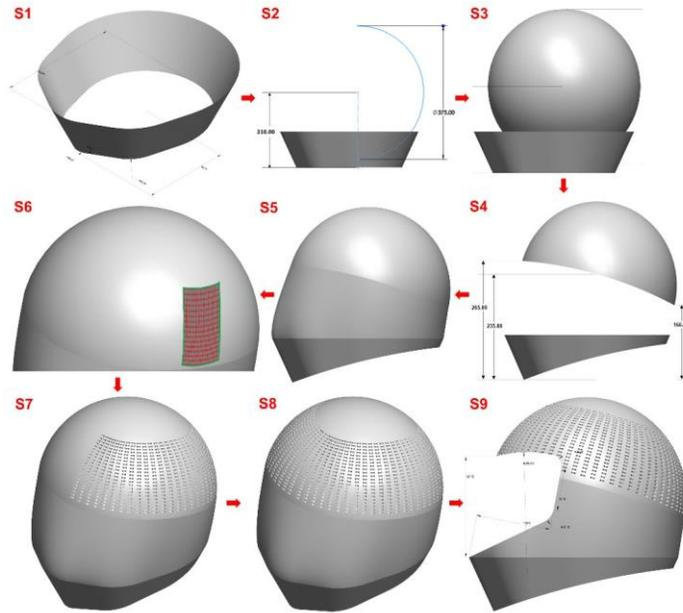
**Figure 4:** 3D CAD model development of the Aux-pore liner using Solidworks™. The step S6 and S7 are as per the proposed methodology and implemented as an automatic module in Solidworks™.
