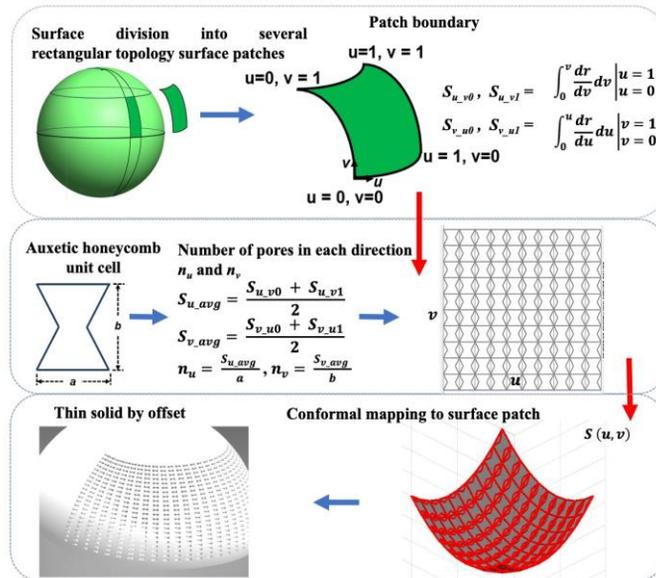
**Figure 1:** Proposed design methodology for mapping lattice structures into thin solids.
