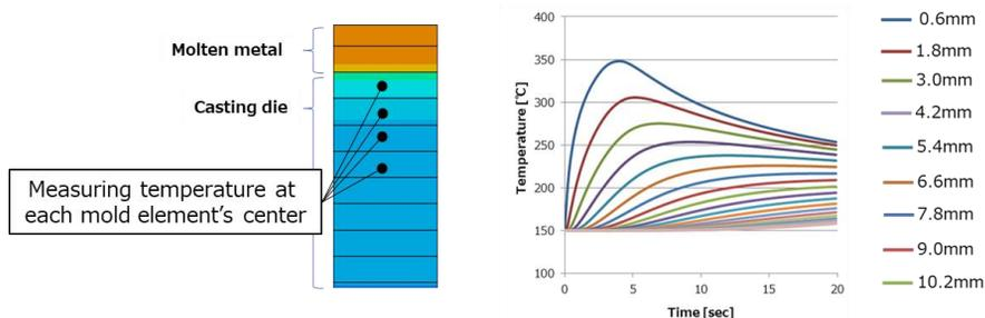
**Figure 2:** (a) Setup of brief simulation, and (b) simulation result of die temperature change over time at each depth from die surface.
