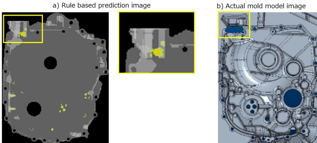
**Figure 12:** Example of (a) rule-based prediction and (b) actual die model.
