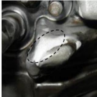
**Figure 1:** Die soldering Image of actual die-casting process.
