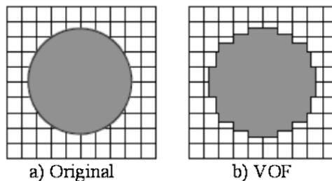
**Figure 3:** Image of differences between (a) Original shape and (b) VOF shape
