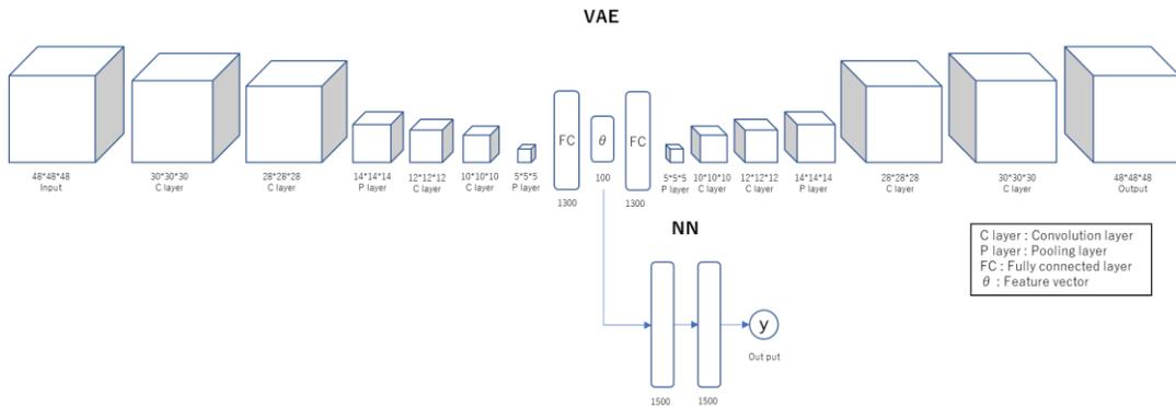
**Figure 9:** Architecture of VAE and Neural Network.
