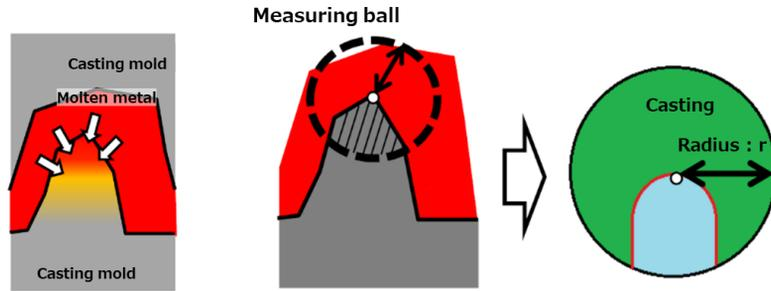
**Figure 5:** Concept of rule-based prediction.
