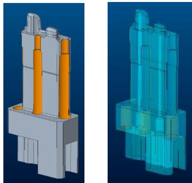
**Figure 13:** Separated die model which has internal cooling circuit.
