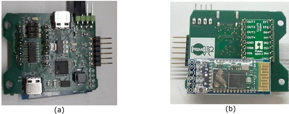
**Figure 2:** (a) Mainboard with (b) Bluetooth (soldered to the backside of the mainboard).
