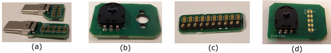
**Figure 4:** The custom-PCBs designed and fabricated for the resistance module: (a) two types of custom-made USB C cables (straight and L-shaped) (b) motor and potentiometer board; (c) female pogo pin board; and (d) potentiometer board for the rotary part.
