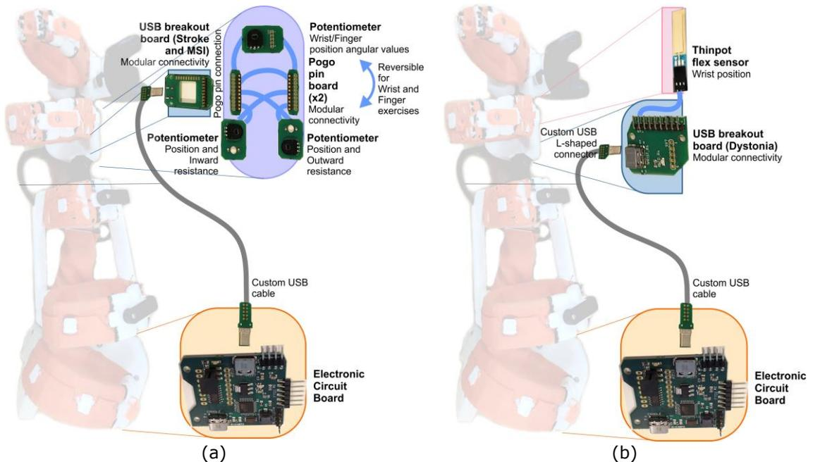
**Figure 5:** Illustration of the electronics components and their corresponding 3D-printed assembly component for the controller for users with stroke and MSIs (a) and users with dystonia (b).
