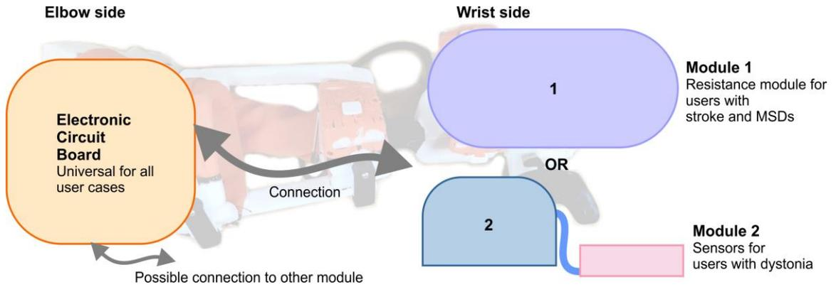
**Figure 1:** Basic bespoke controller configuration.
