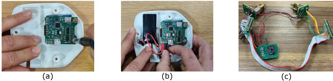
**Figure 6:** Mainboard mounted inside the 3D-printed controller housing (a), lithium battery inserted inside the controller housing (b), and the electronic boards, motors, and potentiometers are soldered together for the assembly process (c).
