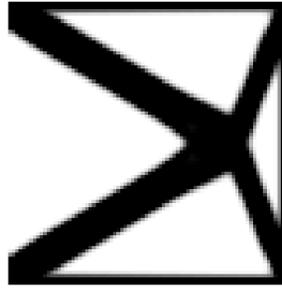
**Figure 4:** Topology optimization results of the traditional variable density method.
