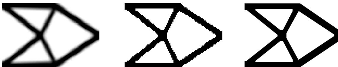
**Figure 13:** Left: Optimization results of traditional variable density method; Middle: Optimization results of partitioned weighted sensitivity filtering method; Right: Optimization results of boundary smooth post-processing method.
