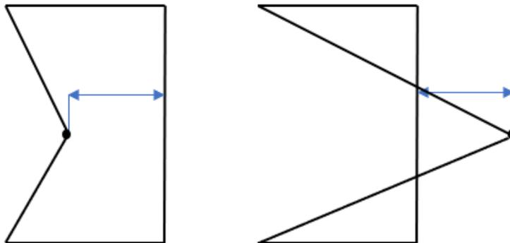
**Figure 14:** A distance between a point and a line. Both sketches are equally valid in a geometrical sense, but only the one to the left will rebuild the CAD feature made from it. The sketch on the right has lines that criss-cross and it will not rebuild
