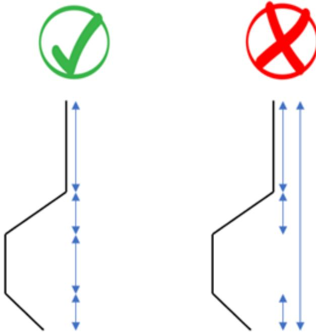
**Figure 13:** Chaining illustrated. The dimensions are stacked along the coordinate axis
