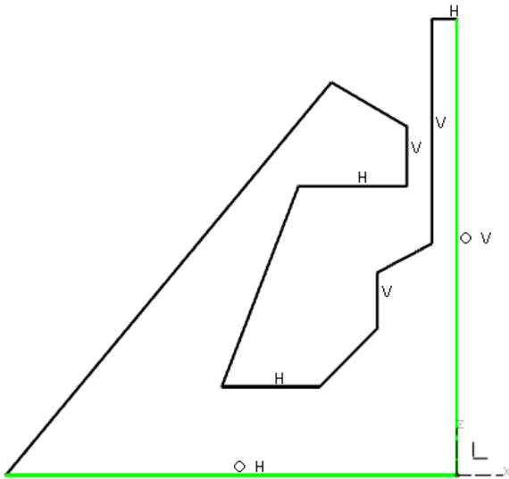
**Figure 5:** The provided sketch for assignments. Black lines = under-constrained, V = vertical constraint, H = horizontal constraint, O = coincident constraint to origin. The green lines indicate iso-constrained.
