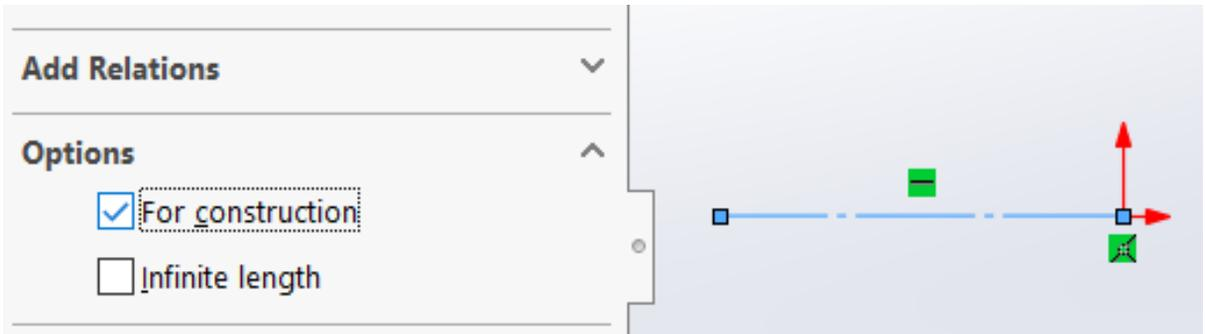
**Figure 17:** In SOLIDWORKS, click on the line, the option to make it a construction line appears in the menu to the left. The line will now not be used to generate any features
