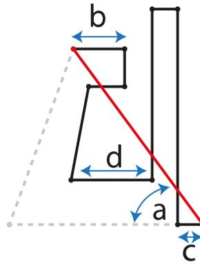
**Figure 3:** Sketch failure due to line flip (red) caused by major change of variable c.
