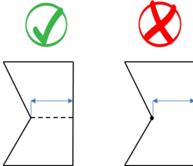
**Figure 15:** Replace dimensions with construction geometry (dashed line) where there are gaps that needs to be constrained
