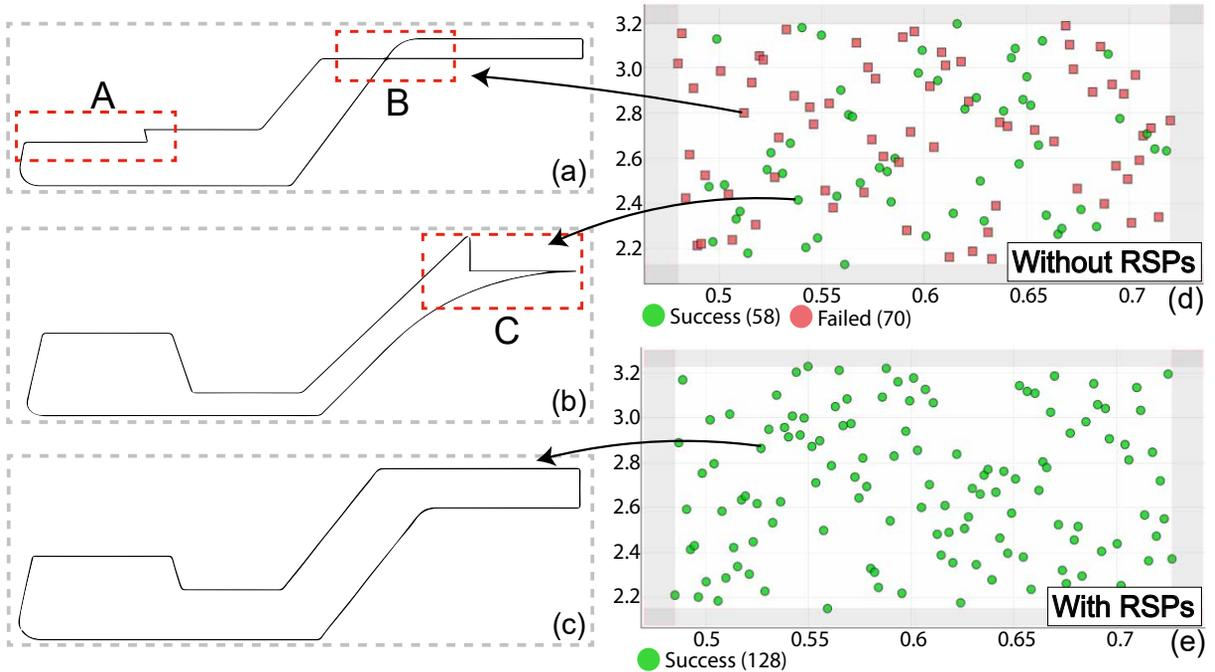
**Figure 10:** The figure shows the industrial sketch 3 with original constraints, affected by  $\pm 30\%$  variation. The middle represents the solution space, where red and green indicate unsuccessful and successful regenerations, respectively. Left side shows an unsuccessful regeneration, where lines overlap and incorrect design intent is present.
