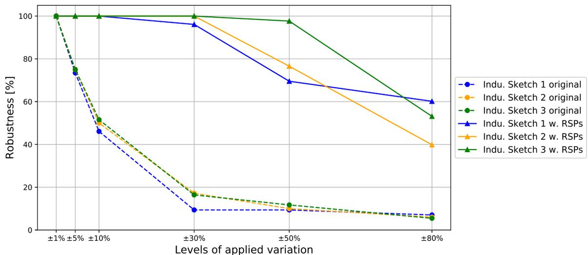
**Figure 9:** Robustness scores of the industrial sketches with and without the RSPs applied.
