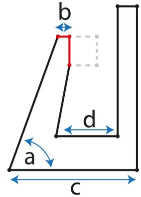
**Figure 4:** Design intent is lost due to incorrect line angle (red).
