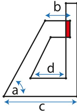
**Figure 2:** Sketch failure due to overlap (red) caused by a change of variable a.
