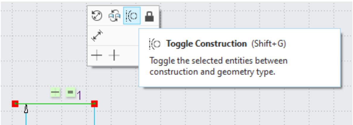
**Figure 18:** In Creo, click on the line, the option to make it a construction line appears in the popup menu. The line will now not be used to generate any features
