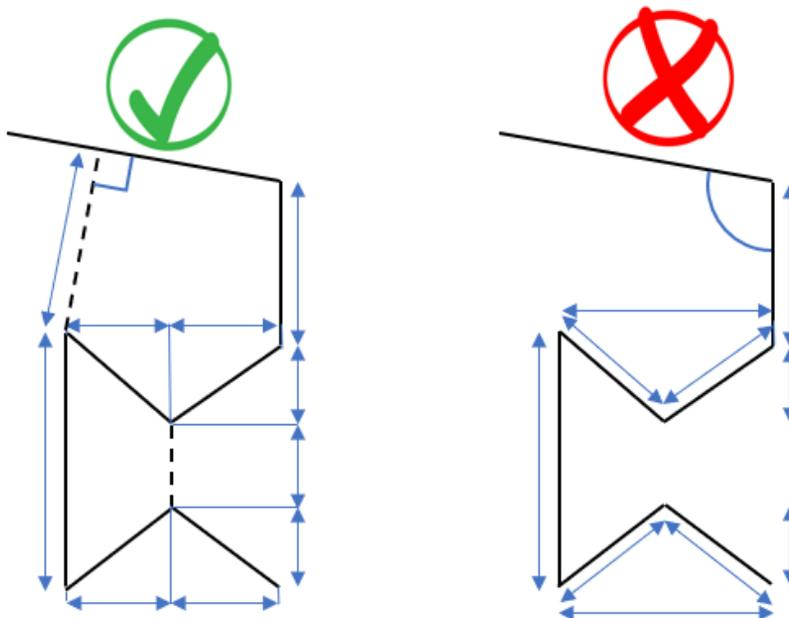
**Figure 16:** Create multiple lines of chaining to deal with multi layer geometry. Create construction lines (dashed lines) to fill gaps in the chaining lines
