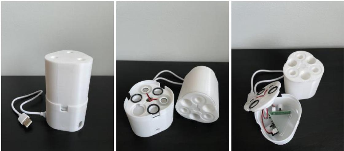
**Figure 4:** Physical prototype of the designed Olfactory Display.
