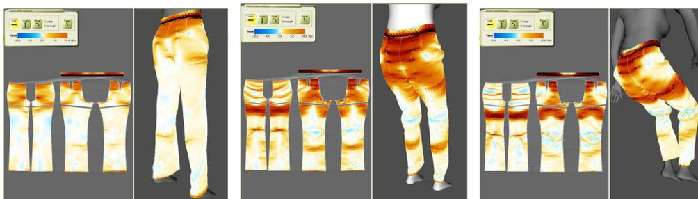
Fig.8: Virtual prototyping: Displaying weft constraints on an animated body (from standing to sitting). Element size is 5mm.
