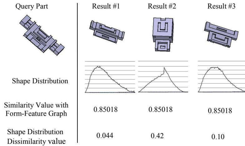
Fig. 8. Limitation of the shape comparison only based the topological information
