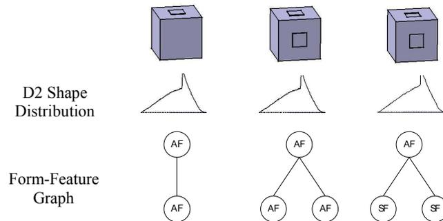
Fig. 9. Shape distributions cannot discern minor geometry variations
