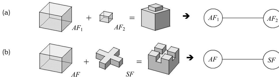
Fig. 4. Generation of an edge in the form-feature graph.
