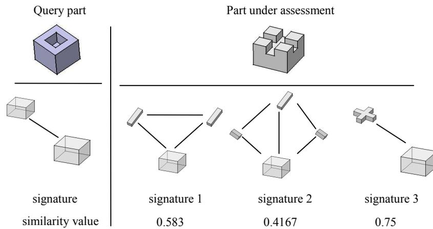
Fig. 7. The proposed approach can eliminate the ambiguity caused by feature interaction
