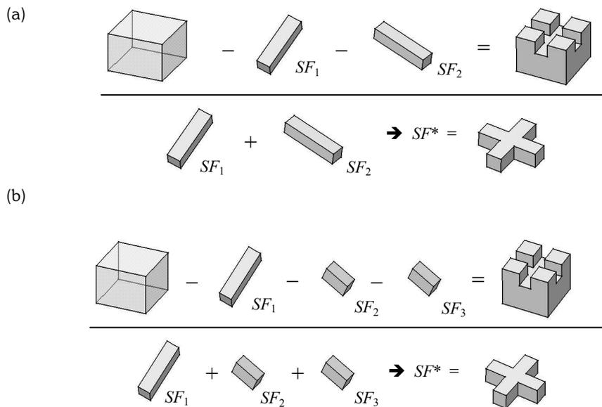
Fig. 3. (a) Generation of SF with feature interaction and (b) with face adjacency.
