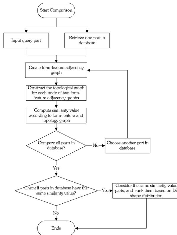
Fig. 1. Part search procedure with multiple shape signatures.
