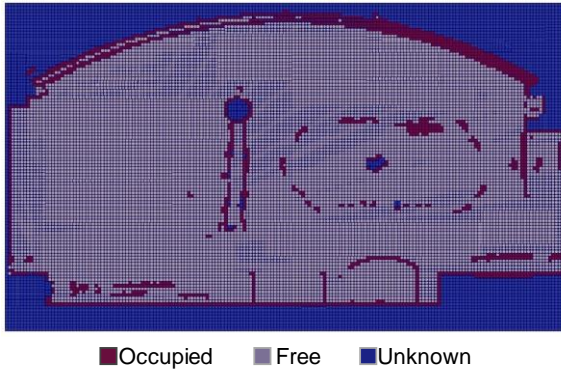
Figure 14: Spatial occupancy classification results before interactive occupancy assignments to the unknown voxel clusters.
