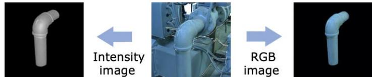
**Figure 6:** Generation of RGB and Intensity images from point clouds.
