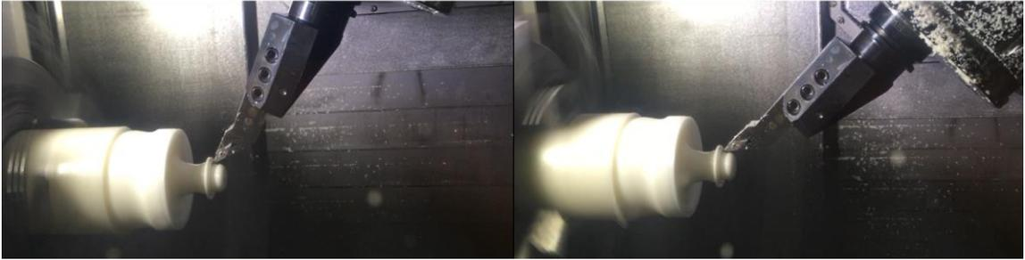
**Figure 22:** Example of part cutting from wax stock. Two positions of tool are shown with clear change in tool angle during operation.
