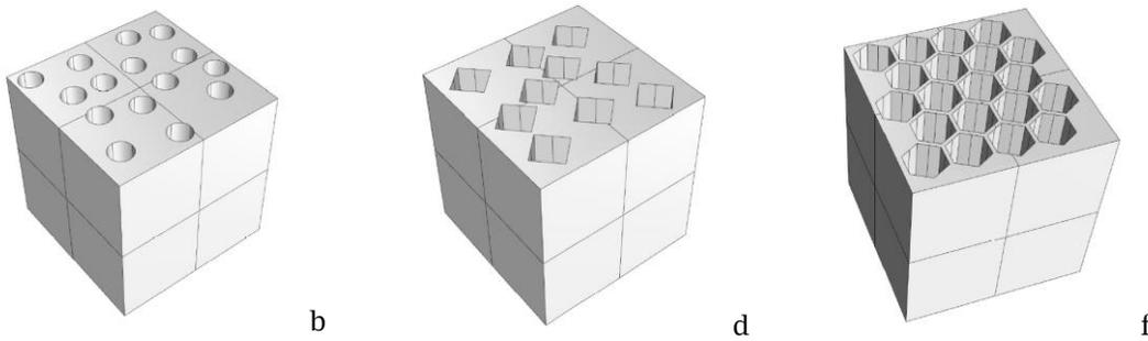
**Figure 2:** Sample data set of CAD models created in Rhinoceros 3D to extract physical properties in COMSOL Multiphysics (a, b) Circular pore shape, (c, d) Rectangle pore shape, and (e, f) Hexagonal pore shape.
