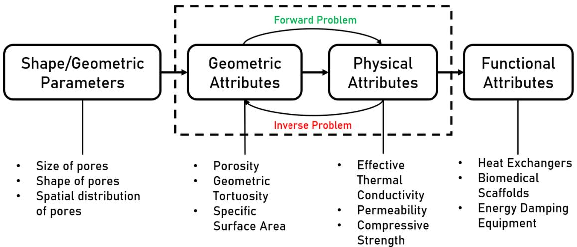
**Forward Problem:** Characterization of physical properties of a porous object (analysis)
