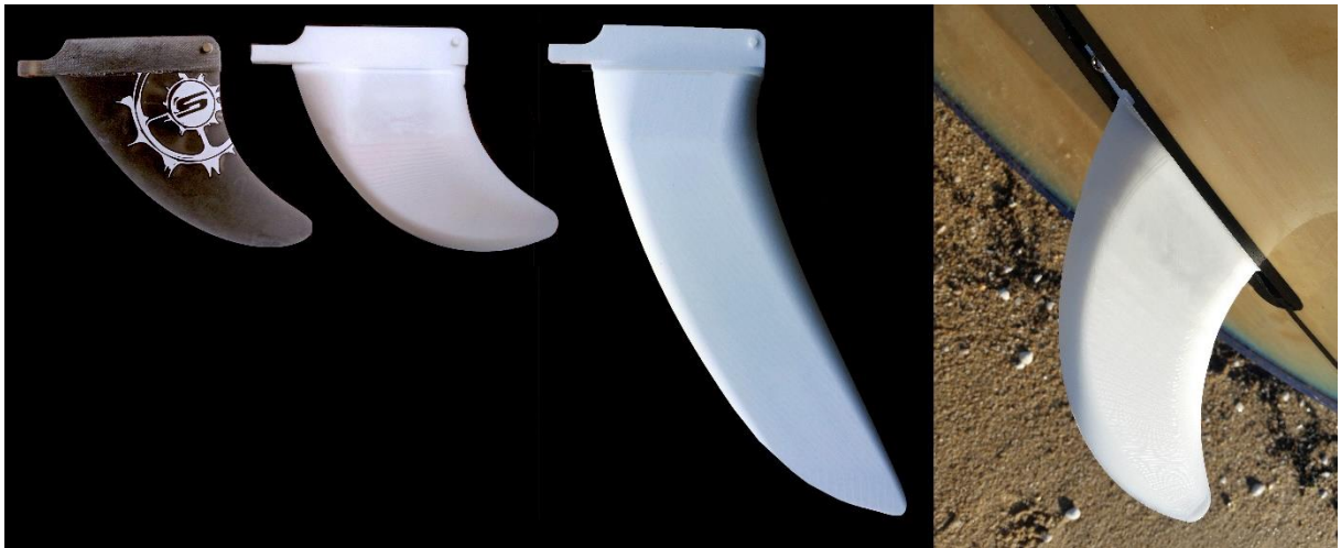
Figure 11. Original 2016 G-Whiz Slingshot SUP center fin (left) compared with a similar version 3D printed using desktop FFF (2nd) and a version 3D printed using Selective Laser Sintering (3rd). Right image shows one of the fins fitted to the SUP board.
