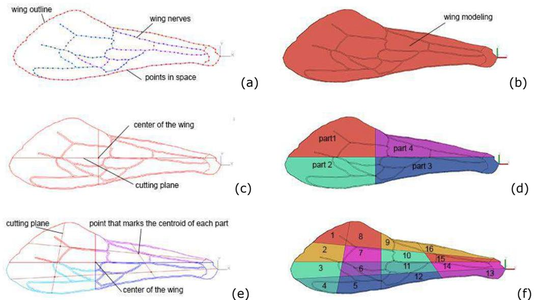
**Figure 5:** Bee wing (a) Points in space, outline and nerves lines, (b) Modeling, (c) Center and two cutting planes, (d) Four parts, (e) Center and six cutting planes, and (f) Sixteen parts.
