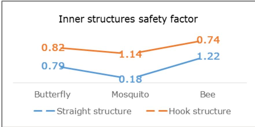
**Figure 24:** Safety factor of inner structure (a) Analysis results and (b) Graphic.
