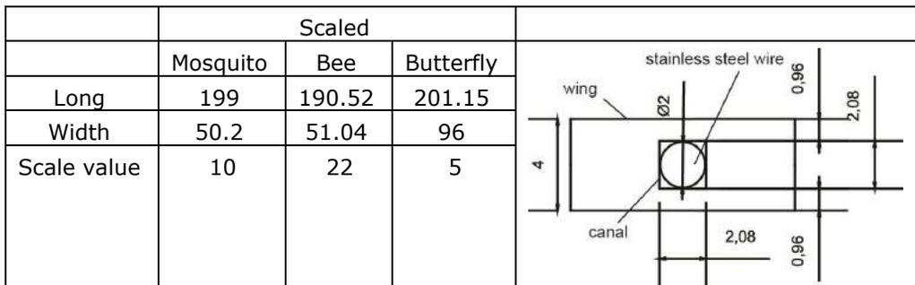
**Figure 8:** (a) Scale value given in mm and (b) Detail of the front view of the wing.
