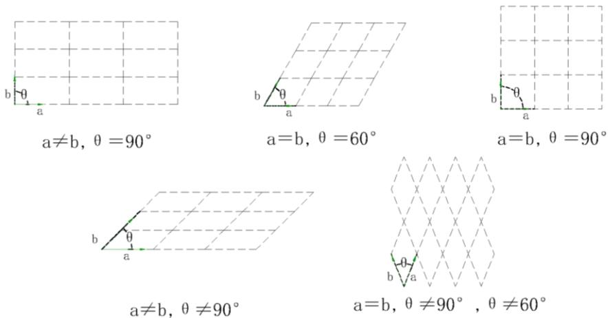
**Figure 4:** Five types of grid systems: (a) Rectangle, (b) Diamond with  $60^\circ$  angle, (c) Square, (d) Oblique parallelogram, and (e) Diamond without  $60^\circ$  and  $90^\circ$  angle.
