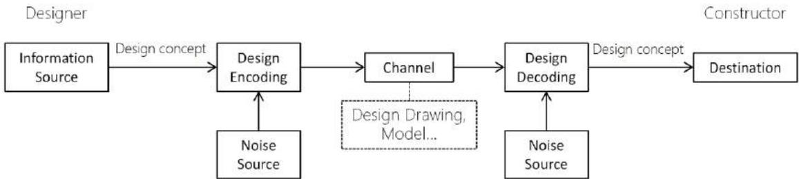
**Figure 6:** The mathematical model of the communication between the designer and constructor.
