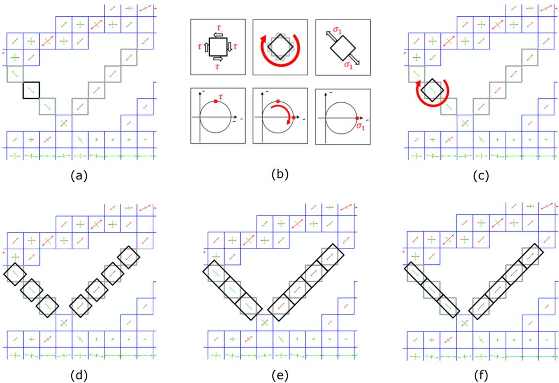
**Figure 3:** Re-orienting, connection and size optimization of the elements.
