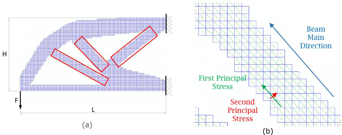
**Figure 1:** Boundary conditions for the case study and result of the process of Topological Optimization.
