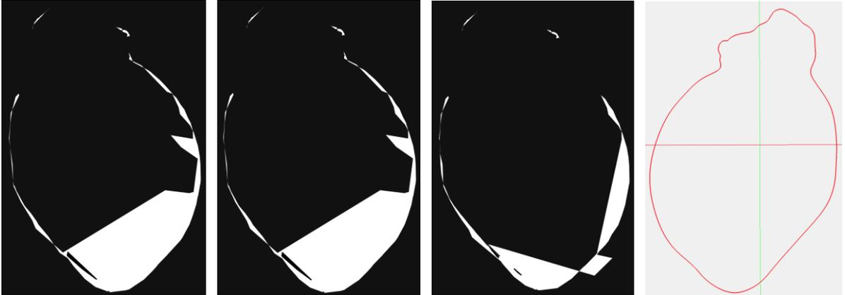
**Figure 9:** Slicing the tessellated head (left three) and the precise NURBS model (right).
