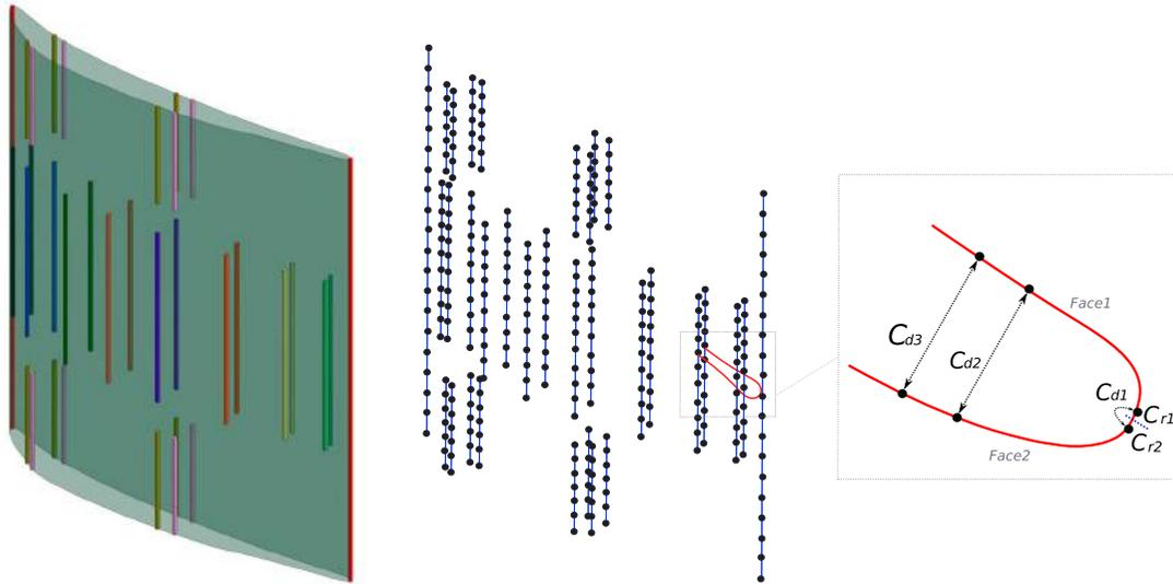
**Figure 9.** Left: Constraint visualization from the STEP file; Right: Constraints computation on the testpoints
