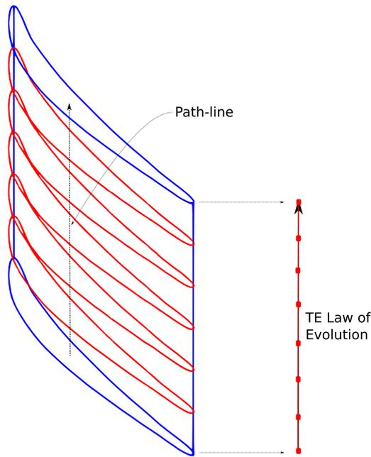
**Figure 6.** Blade skeleton and TE law of evolution in the 3D domain
