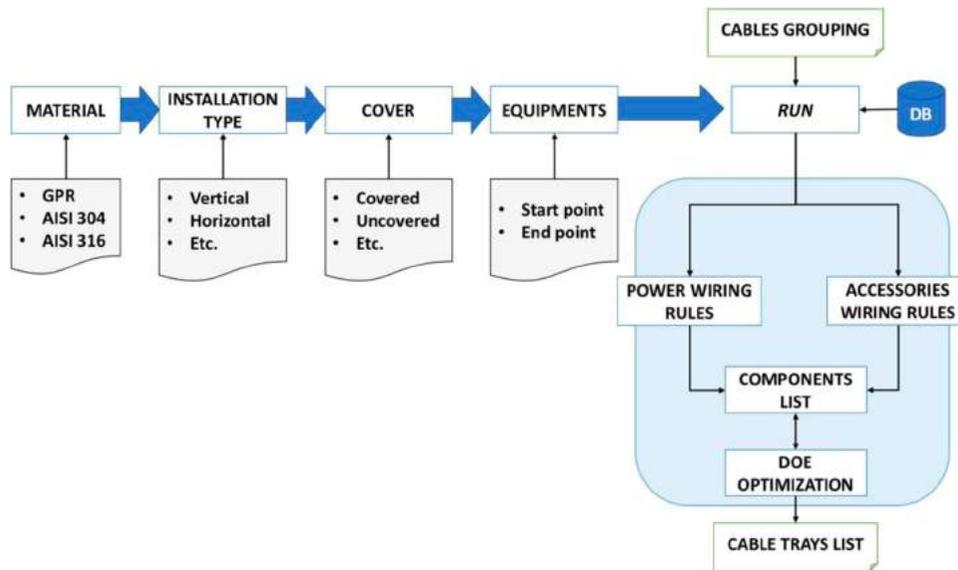
**Figure 2.** The workflow related to the *CT SIZING OPTIMIZATION* tool.
