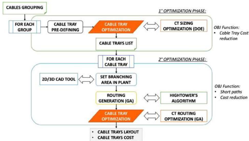
**Figure 1.** The proposed design methodology for the cost optimization of electrical cable trays.
