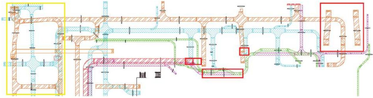
**Figure 6.** Not optimized routing of the cable trails reached in a traditional way.
