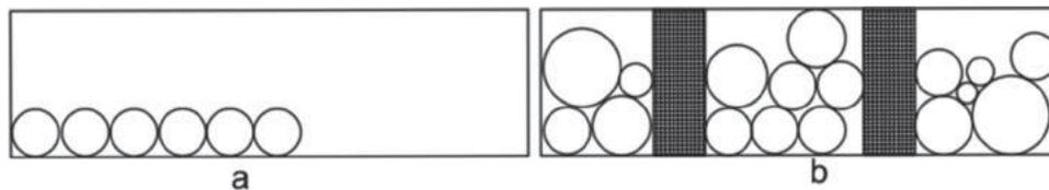
**Figure 3.** Possible cables arrangements: (a) linear arrangement for power cables, (b) volumetric arrangement for instrumental cables.
