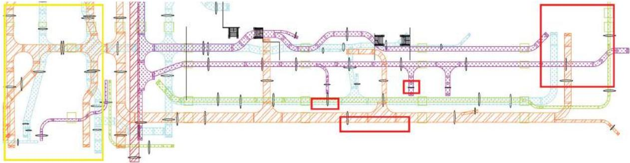
**Figure 7.** Optimal routing of the cable trails reached by the proposed methodology.
