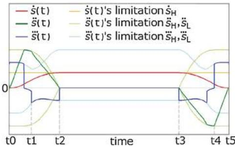
**Figure 2.** A time optimal driving pattern on a circle path.
