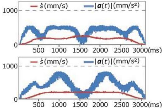
**Figure 7.** Driving results of Fig. 6 by using time optimal pattern (top graph) and using modified constant velocity Cam pattern (bottom graph).
