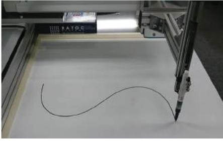
**Figure 6.** Plot s-curve by a manipulator.
