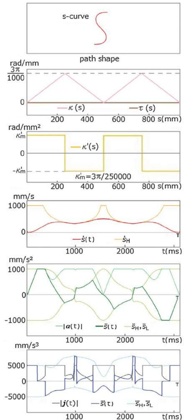
**Figure 3.** Time optimal driving pattern on a S-curve path of  $h = 1000$  mm.
