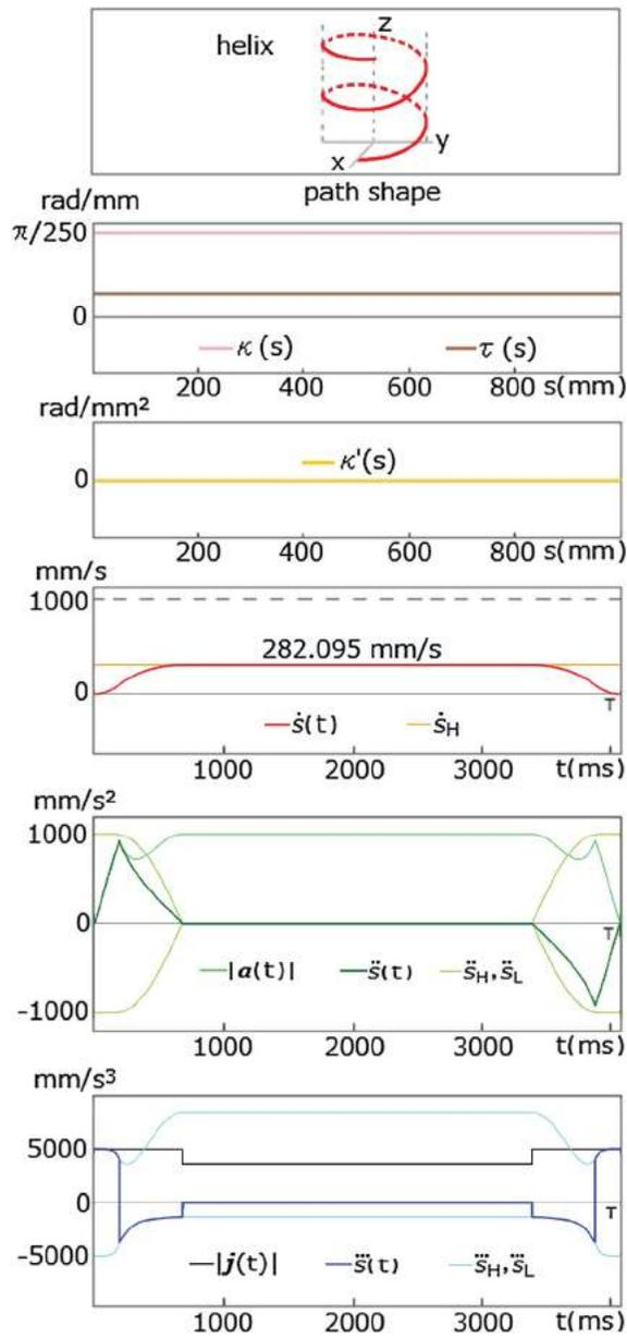
**Figure 4.** Time optimal driving pattern on a helix path of  $h = 1000$  mm.
