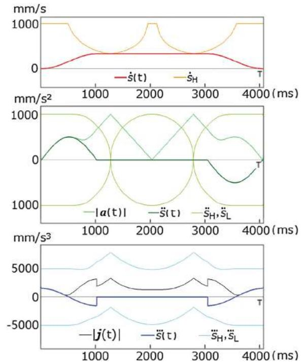
**Figure 5.** Modified constant velocity driving patterns on the s-curve of Fig. 3.
