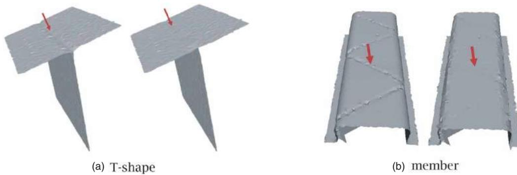
**Figure 6.** Dent removal result.
