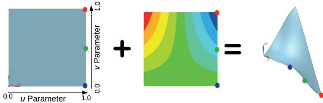
**Figure 4.** The preliminary surface and displacement data create the mode shape surface.
