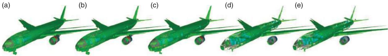
**Figure 4.** Five levels of detail of Boeing 777 model. The numbers of triangles and vertices (triangle/vertex) are: (a) 38.0M/25.0M; (b) 26.6M/17.5M; (c) 15.1M/10.0M; (d) 7.4M/5.0M; (e) 3.7M/2.5M.
