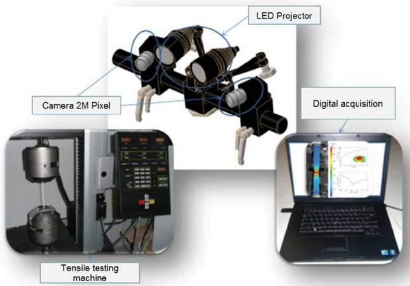
Figure 5. DIC measurement Device.
