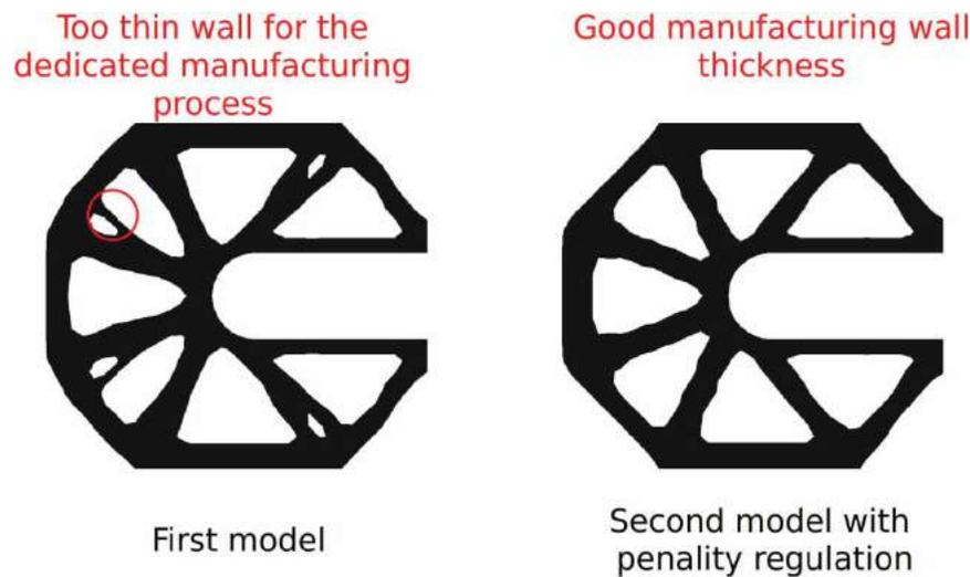
**Figure 3.** Test-case on C-CLIP for the management of too thin walls.
