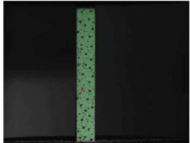
Figure 6. DIC measurement example.
