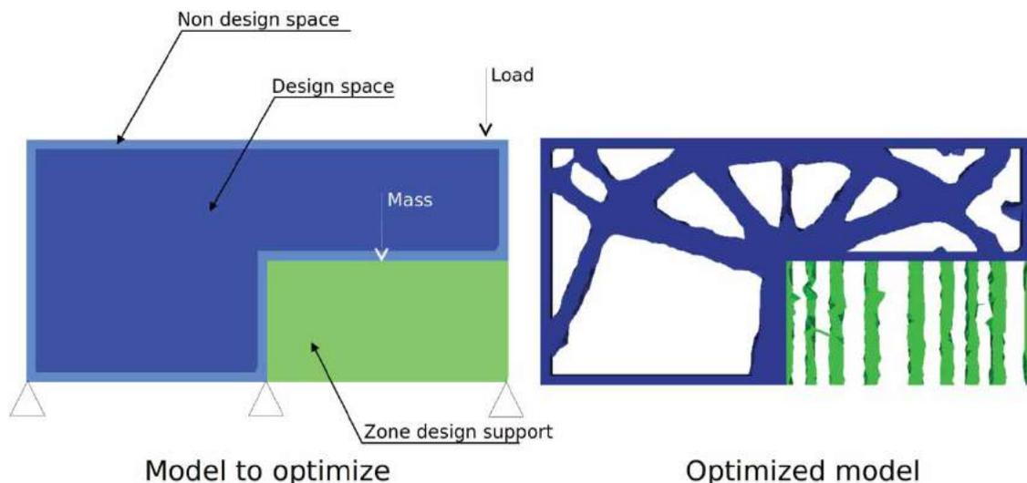
**Figure 1.** Simple example of part and support optimization.
