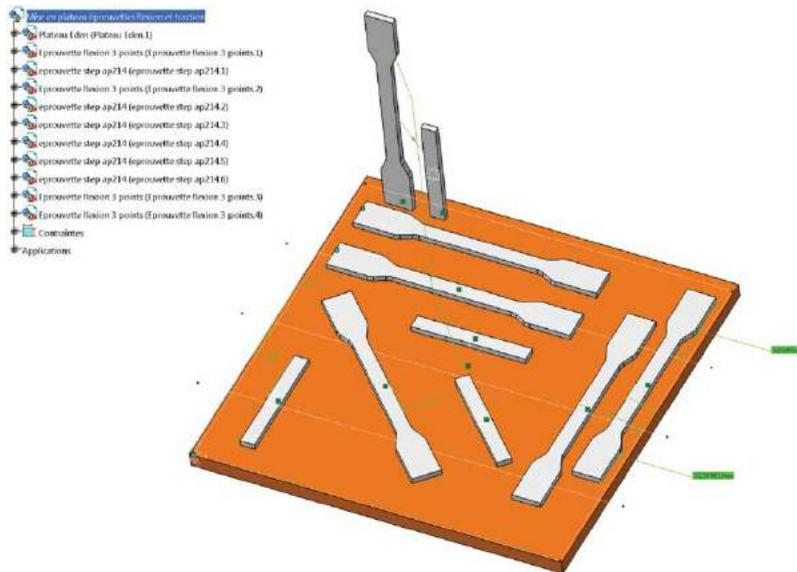
Figure 4. Tensile specimens orientation.
