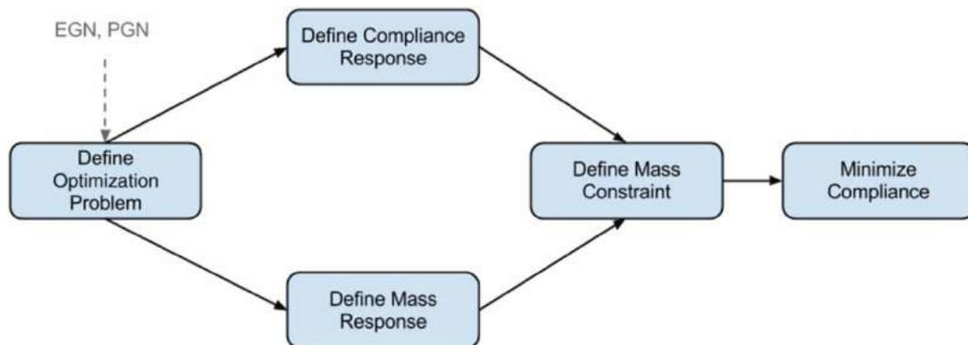
**Figure 9.** Mass scenario for topological optimization in AM.
