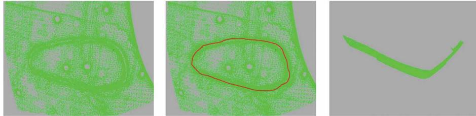
Fig. 6: Example for boundary point detection: (a) front view, (b) ideal boundary, (c) top view.
