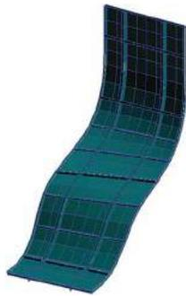
Fig. 36: Fine FE mesh of the ship hull surface structure.
