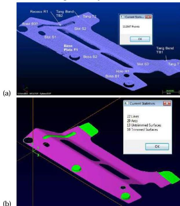
Fig. 3: (a) Stamped panel reconstruction points and (b) final geometry.
