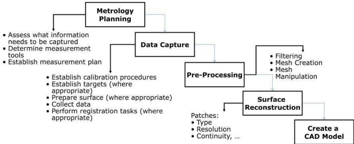
Fig. 1: Standard process flow for reverse engineering.
