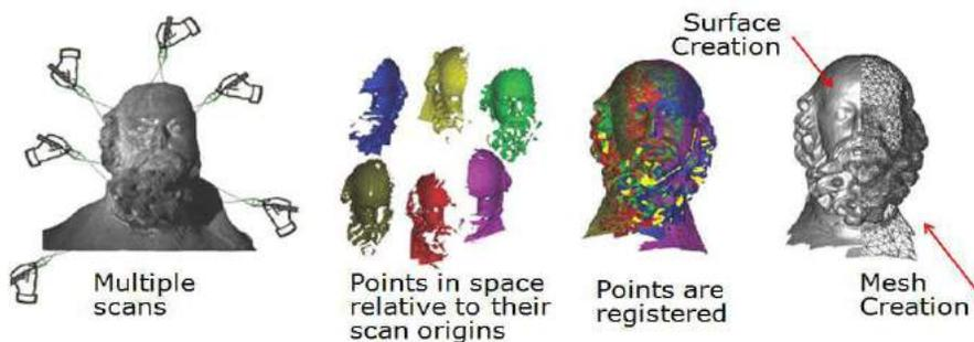
Fig. 2: (a) Multiple scans, (b) point cloud data, (c) registration and (d) surface generation for a sculpture adapted from [10].
