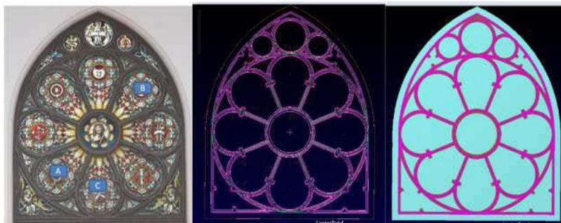
Fig. 10: (a) Rose window digital image, (b) wire frame geometry and (c) solid model reconstruction.
