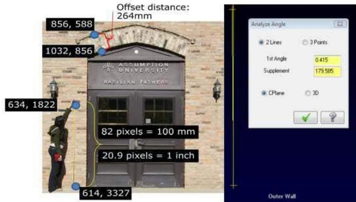
Fig. 11: (a) Digital image, scale, and initial calibration and (b) orientation angle.
