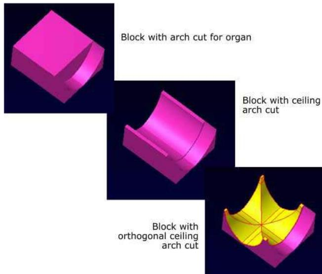
Fig. 17: Decomposed method for creating the chapel ceiling.
