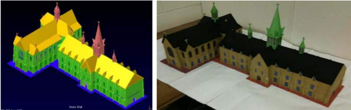
Fig. 20: Completed CAD model and completed build assembly.
