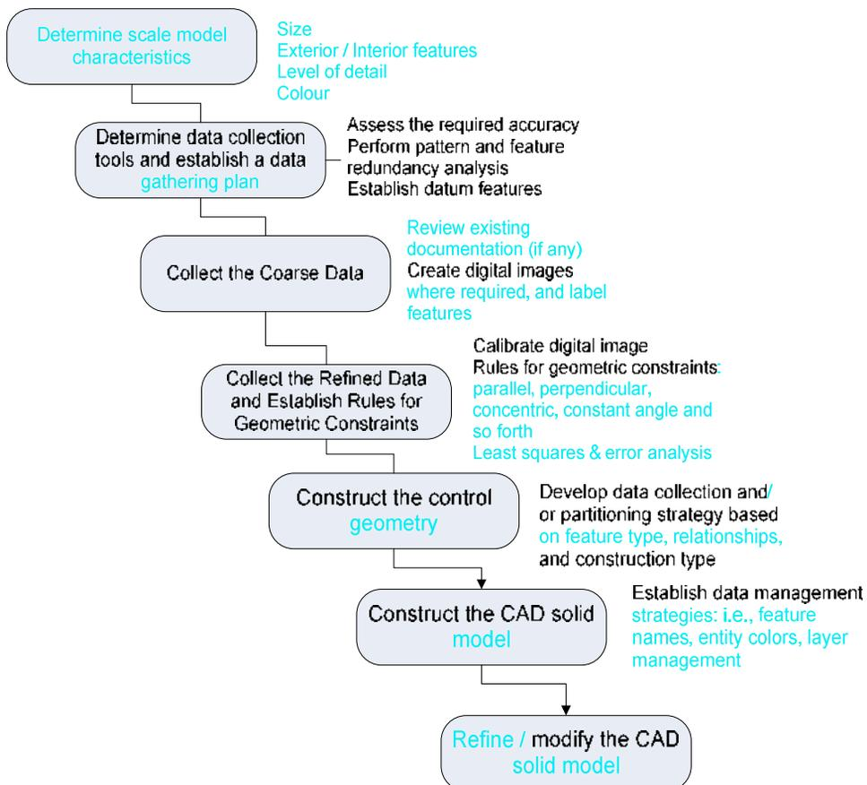
Fig. 5: Process flow for reverse engineering an architectural building.
