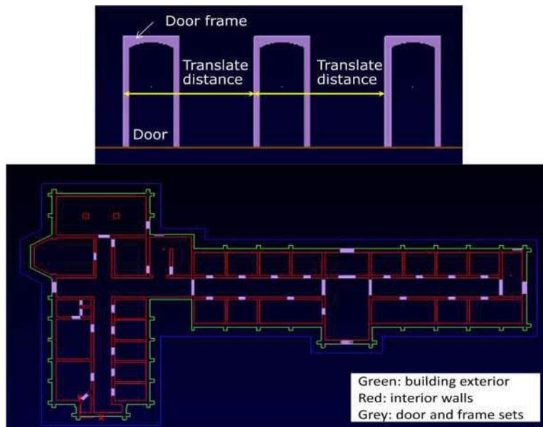
Fig. 12: (a) Door and frame, and (b) first floor base line geometry.
