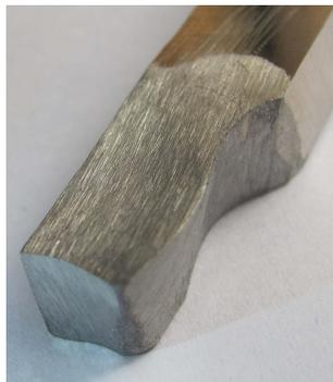
Fig. 7: SPCT with free-form cutting edge.
