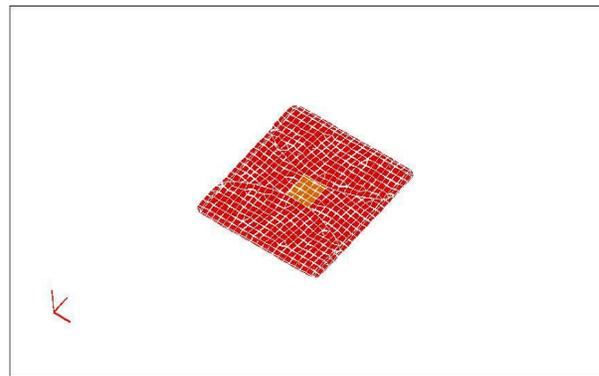
Fig. 7. The generated mesh on the airbag folded with SAFE EDITOR
